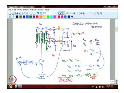
We have the supply V in there is a forward converter transformer, which is connected in this fashion to a power semiconductor switch. I am indicating the power semiconductor switch by a B J T; however this B J T could as well be an M O S F E T or an I G B T.
