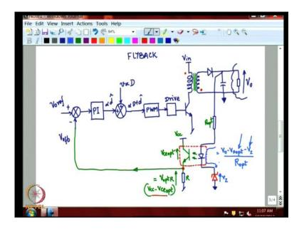
So, before that let us clean up some of these things here. Yes and this. So, here the new component that I am going to add is a senor and then, you are connected to. Now, choose senor such that these two are having an opposite temperature coefficient. So, this is having a positive temperature co efficient and this should have negative temperature co efficient, so that there is compensation.
