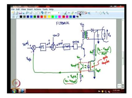
So, if we take the fly back convertor, it is of this form. You have the fly back transformer which is also actually an inductor, where I am using this b j t or i j b t. You can actually replace it with mosfet, i j b t or b j t or let say, you have this drive and this comes from
