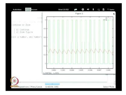
So, this is the red waveform is the inductor current waveform, and the green waveform is actually the pulse width modulated waveform that has been generated to achieve that steady output voltage of 20 volts. So, this pulse width modulated waveform 0 to 1 is actually the gate drive signal which is given to the boost convertor switch and you see this triangular waveform in the current waveform in the inductor as discussed in the analysis of the boost convertor, ok.
