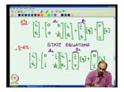
And from here we started developing the state equations during d t s time this was the state equation that we developed and during 1 minus d t s time this was the state equation that was developed.
