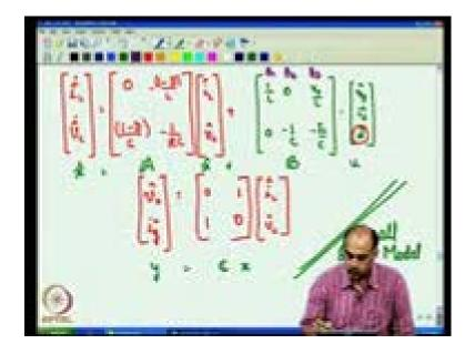
If we consider the b matrices columns, so let us say b column 1 b column 2 b column 3, so b column 1 we used for Vg b column 2 is used for I z b column 3 is used for d in trying to obtain for the heat transfer functions.
