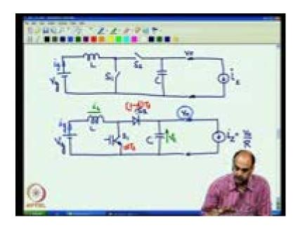
This is the boost converter which we discussed, it contains the input source v g input current i g l two switches s 1 and s 2 c and load current I z. This is also representable in terms of switches here it can have a IGBT here, or diode as these two switches IGBT switches during v t s time and the diodes comes into action during 1 minus d T s time.
