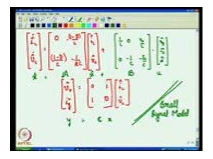
Which is of this form so either you could have this or this. The output equation also could be combined together in the following manner you could have I g hat like hat 1 0 so this also results in the same output equation y is equal to c x x dot hat equals a x hat plus another matrix. Let us say m d hat plus or we will put it b 1 d hat plus b 2 V g hat plus b 3 I z hat you could also combine the three inputs in the following manner. So what we shall do these three inputs.
