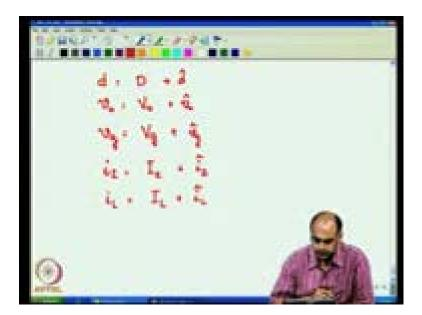
We can now try to get these small signal models so these small signal model is obtained by substituting in the average signal model for every variable a steady state part and A small signal variation about the steady state or equilibrium point v naught is equal to v naught plus v naught hat, so the variation about the.
