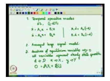
So, summarizing the process we first from the circuit depending upon the temporal modes operative modes that is d t s 1 minus d t s timed duration split the circuit and obtain the each models for each of the temporal modes. That is you have a 1 x plus b 1 u and that would be extra and then you would have a 2 x and b 2 u then you can combine them by making a averaging in this fashion.
