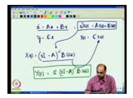
So let us see now how we go about getting the transfer function from the state spares model you know that the state spares model is given by A x plus B u and y is equal to c x
