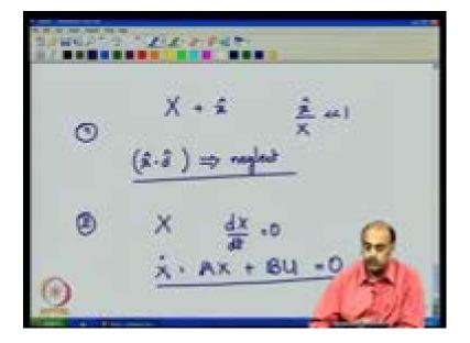
We said that the steady state part is very large compared to the small signal part. Small signal part is very small compared to the steady state part. Therefore, if you have a term which is multiplication of two small signal part then we can neglect this term, because x hat itself is very small compared to x. So, in the normalized form a very small number less than 1 into a very small number less than 1, we are trying to neglect it, that it is not, so to significant.
