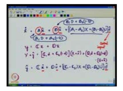
Now, this A matrices is nothing but A 1 into upper case D plus A 2 into 1 minus upper case B. Only the steady state portion comes into the picture here. Likewise, here also you have B into upper case D plus B 2 into 1 minus upper case D. So, that would be the expanded form of this, this having come from the simplification, simplification of this equation.
