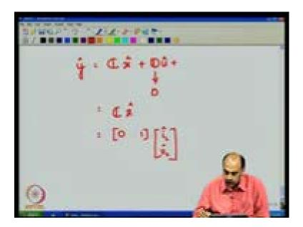
So, this becomes the small signal, this becomes the small signal model which gives deviations about the operating point. All are deviations about the operating point, every variable here use this deviation about the operating point. So, the key here likewise the output variable, which in this case is trivial case where you have y hat, which is equal to C x hat plus D u hat plus du d you have, but in this case d 0.
