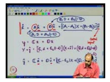
So, there for the average, from the averaged model, we obtained the small signal model by applying these, by applying values to this equations like this.
