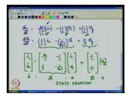
Now, these are the two equations which, which have been developed from the two dynamic components, and these basically form the state equation if they are re-arranged in a proper manner. So, let us do the re-arrangement by copying this equation set into a fresh page. Now, this equation set, we will arrange it in the form of a matrix.
