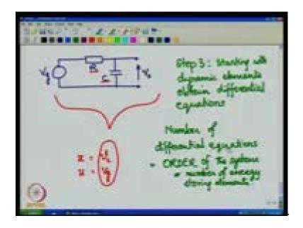
So, considering these two variables you have just these two variables the whole system has been represented with just this to these two variables. Plus the parameters the fixed or the constant parameters that define the system, this case R and C, these are the only variable system, we need to use that from to use only this two. Now, let us look at the the system based on these two variable only. Now, take start always with the dynamic equations.
