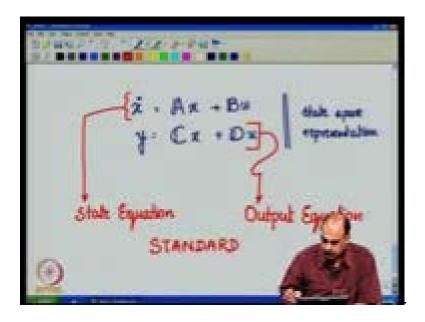
So, the state space that representation is given in this fashion. x dot, which is equal to A x plus B u and y, which is equal to C x plus D u. All physical systems all linear physical systems can be brought into this state space representation. This is also called the state, let me write it down here. This first equation is called the state equation. The second equation is called the output equation, so this is the standard form, which is used for representing all linear physical systems.
