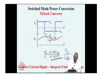
And if we combine these 2 quantities, we get the ratio of the ripple current to the average current in the inductor, which is 1 minus D whole square T S by 1 by R T S is the switching period and 1 by R is the time constant of the load and the inductor. And if this ratio switching time is very much small compare to the time constant of the converter then this ripple will be small.
