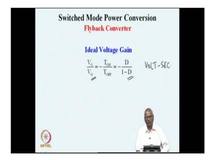
So, practically now, we have done the ideal as well as the non ideal steady state analysis of this converter. And we see that the ideal voltage gain of this converter is V naught by V G which is minus D by 1 minus D. This was obtained by applying the volts second balance on the inductor; this was our method of evaluating the ideal voltage gain.
