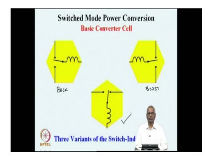
We had also seen that this basics cell could be used in 3 different variants to form different basic power converter cells. The first one and the second one we had already seen all the Buck power converter, the Boost power converter and what we will be seeing today will be the third converter, which goes by the name of Buck boost or fly back power converter.
