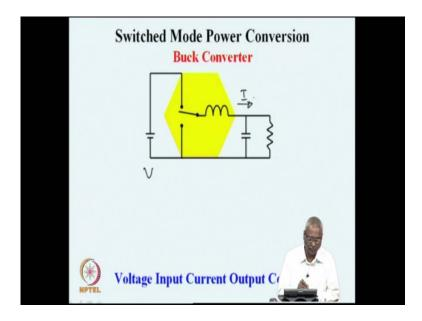
In the first type of power converter the input was a voltage and output was a current, we could say that this is the voltage input current, output power converter.
