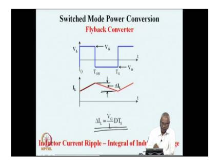
And if we integrate this voltage, we will see that during the on time this positive voltage V G results in an increase in the inductor current during the off time the negative voltage, that is applied across the inductor results in a drop in current. Understudy state the rise in current during on time is a same as drop in current during off time and we can write this delta I l or the ripple current as the slope V G by l and multiplied by on time which is D
