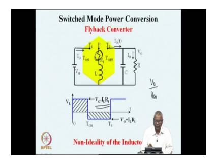
The inductor has another non ideality, which is a resistor. So, no inductor can be with 0 resistances as we are using a conducting wire to wind the inductor it has a resistance
