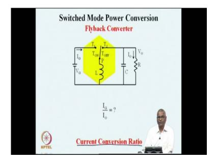
The ratio of I G by I naught is found simply by current conversion or this is defined as a current conversion ratio and this can be found out by averaging the output current.
