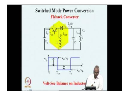
We keep account of the voltage drop volts second balance. And the inductor is now V G supply voltage minus the device drop the transistor drop during on time. And similarly, the output voltage plus the diode drop during the off time.
