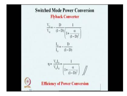
We can also say that, this correction factor is the same as efficiency; the efficiency of power conversion is the same as this correction factor 1 by 1 plus alpha by 1 minus D whole square. Interestingly this correction factor is identical for the boost converter as well as the fly back converter.
