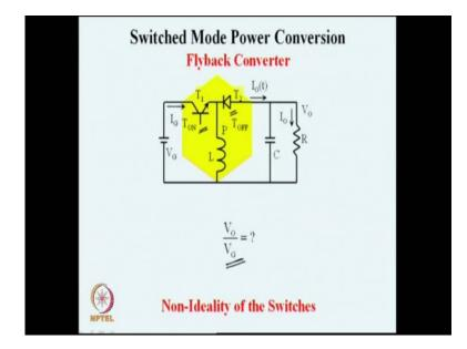
The non ideality in the converter, on account of the switches having non zero drops can be found out by finding out, what is the voltage drop in the switch? When it is on and what is the voltage drop in the diode? When the diode is conducting. If we apply these non idealities, we will come across a different ratio of V naught by V G that we apply gain the same principle, which is the volts second balance.
