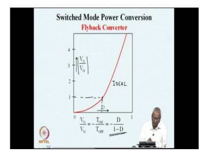
This can be plotted this ratio; this function of D of this V naught by V G can be plotted as a function of D. And you see that it starts from 0 when D is 0 and it goes to infinity when D is 1 and this would be the ideal gain characteristics of the fly back converter. So, as D varies from 0 to 1, the gain varies from 0 to infinity, when D is equal to 0.5 the gain will be 1, when D is 0.5 again is 0.5 divided by 0.5 which is 1 input and output voltages will be equal.
