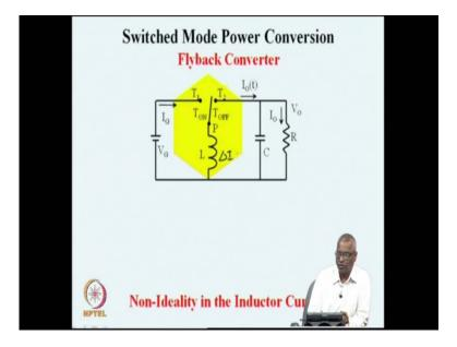
The non idealities are the inductor current ripple and the capacitor voltage ripple and this is found out the current ripple or delta I in the inductor is found out by integrating.
