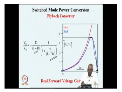
So, on account of this correction factor, V naught by V G now is not just D by 1 minus D, which is shown by the red color line here it is getting modified by a Correction factor. And once the correction factor is included, the gain of the converter drops to 0 has you
