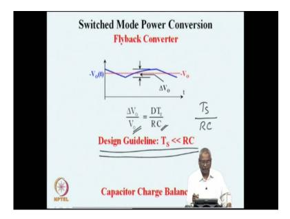
Again it is good to represent it as a ratio normalized it on the output voltage. So, this is duty ratio times switching period divided by the load time constant, and the design guideline to keep the unwanted ripple on the output, because clear from this, that if the switching period T S is very much less than the load time constant RC. Then we will have low ripple and that could be our design guide line and this is obtained by the capacitor charge balance.
