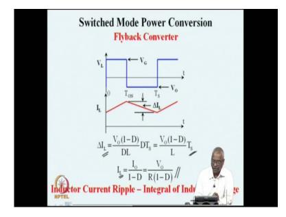
It will always good to represent the voltage, the voltage ripple as a fraction of the current through the inductor. The current ripple as a fraction of the current through the ripple and when we do that this I l is a related through the output current V naught by R divided by 1 minus D delta I l. We had just now found out V naught by l into 1 minus D T S.
