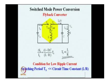
And that could be one of our conditions for design of the converters. So, we can say that for low ripple current as the performance of the inverter of for the inductor current to reach the ideal condition, it is necessary that this inequality is met better T S. If it is becoming a smaller and smaller fraction of l by R then our inductor ripple current will go towards 0. So, the design criterion is that the switching period T S must be very small compare to the circuit time constant l by R.
