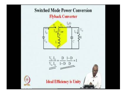
Similar results, we have seen for the buck converter and the boost converter and we are seeing the same thing following similar lines of analysis and the efficiency is given by the ratio of voltage conversion and current conversion, which is 1 and this is what we expect in the ideal case.
