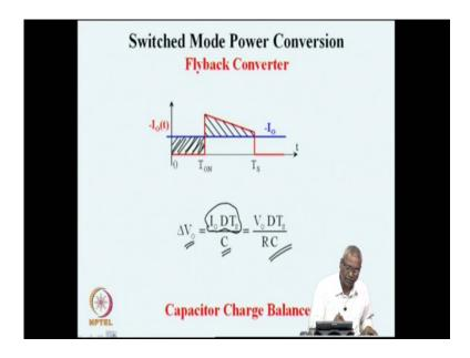
So, we find that I naught into D T S is the area here and this area multiplied or this I naught multiplied by D T S is the current taken from charge taken from the capacitor divided by the value of C will give us delta V naught. And that is output voltage multiplied by on time divided by RC time constant of that.
