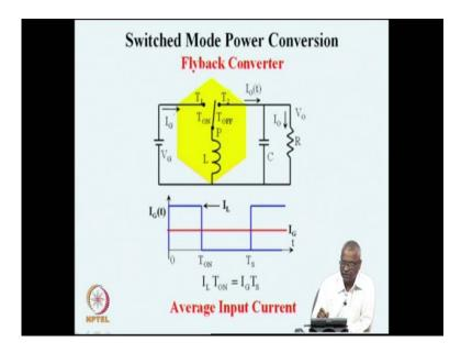
We see that this I naught t the, is the same as the inductor current during the off time, and inductor current is I l it does not have any ripple. So, this current during the off time is flowing through the load. And so the average of that is I l into T OFF which is equal to I naught into T S and we can say that I l is I naught into T S by T OFF, this is the average input current. In the similar way, average input current can be seen as during T ON I l is
