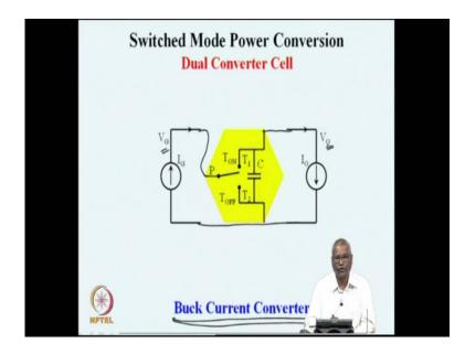
And it is possible to connect this as a buck current converter. And if we had seen the previous cell as a converter, the buck voltage converter where it converts V G to V G to
