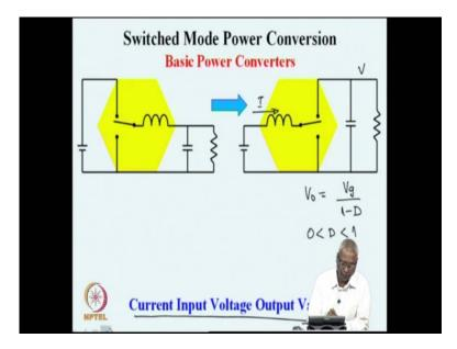
And the second converter had current as the input and voltage as the output. And we could say that as a current input, that voltage output power converter, which boosts the output voltage in this converter V naught is V G divided by 1 minus D where D is varying in the ratio of 00 to 1. And this converter was boosting the input voltage. The input current is stiff and output voltage is stiff and we could call this as a current input and voltage output variant.
