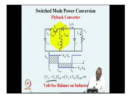
And if we now take the volts second balance, we find that if we see that V naught plus V D that is because the polarity of V naught is negative. On account of that, this ratio the on time voltage is algebraically V G minus V T into T ON off time voltage is algebraically V D into T OFF.
