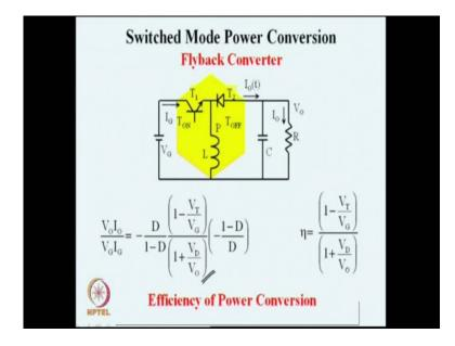
And when we multiply these 2 terms we get our efficiency which is 1 minus V T by V G divided by 1 plus V D by V naught. The method of evaluating the voltage gain, current gain, and the current ripple in the inductor the efficiency on account of the switch drops they follow the same method; volts second balance on the inductor, integrating the inductor voltage to get the inductor current and so on.
