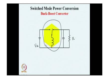
To, what we had seen in the past, in the past 1 hour is to look at this buck boost converter of fly back converter has made up of a converters cell connected to a voltage source and connected to a load.
