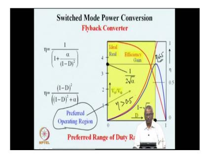
And so we would like to operate at the lower end of duty ratio where the efficiency is more than 0.5 what you see here and the yellow region here is the region where the gain is in the increasing range where it has not reach the maximum. So, in that region gain is more than 0.5 and on the other region in the next region, the efficiency is less than 0.5 and that is not our preferred region, our preferred operating region is the region where efficiency is greater than 0.5. So, what is shown here?
