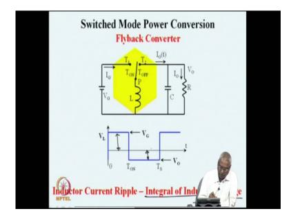
The voltage across the integral of inductor voltage will give us what is the current ripple the inductor is applied voltage of V G during on time and V naught during off time.
