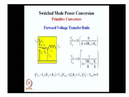
And if we combine these things and find out the volts second balance, this V naught by V G applying this average voltage across the inductor being 0, V naught by V G now has the ideal ratio D multiplied by a correction factor. Here also, the correction factor is less than 1, it is the load résistance divided by load résistance plus duty ratio time source résistance plus the inductor resistance and this number will be close to 1 but, less than 1 and that is what we notice here.
