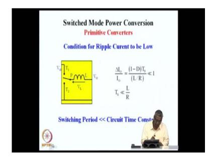
So, if the non-ideal condition of ripple current has to be very low then, we can say that this non-ideality which is delta I naught by I naught which is 1 minus D T S by L by R has to be very much less than 1 or we can alternately say that the switching period T S has to be very much less compared to the circuit time constant L by R. This is one of the conditions for the non-ideality to be negligible or for the converter to perform as close to the ideal as possible.
