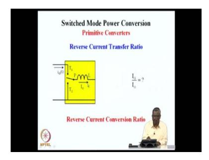
The second performance measure in any converter is the ratio of the average input current in relation to the average output current. The reverse current conversion ratio is the ratio of the average value of this I G of t divided by the output current I naught. This ratio is called the reverse current conversion ratio.
