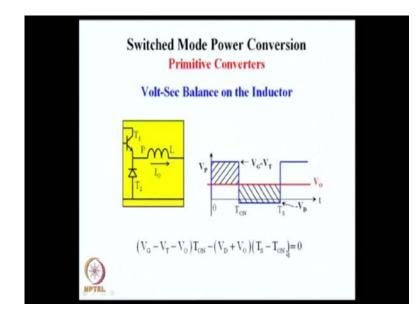
This volt second balance is nothing but the average voltage across the inductor in one cycle. That is also referred to as volts second balance and when it is evaluated it is V G minus V T minus V naught which is this area of this hatched region this multiplied by T ON. Similarly, this during the OFF period minus V D minus V naught multiplied by the OFF period.
