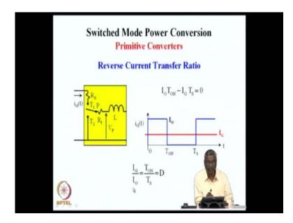
And just as before, the current conversion ratio is not affected by the presence of R S or R L because these are all series non-idealities. When we evaluate the average current it continues to be as before. And so, the ratio of I G by I naught is still the same as duty ratio.
