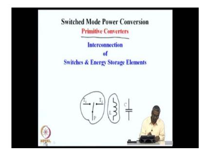
What we are going to study now in this session is about a primitive converter and this converter will consists of a single switch and one inductor. How we connect them together, following certain principles on circuit theory in order to carry out the power conversion function efficiently is what we are going to do in this lecture.
