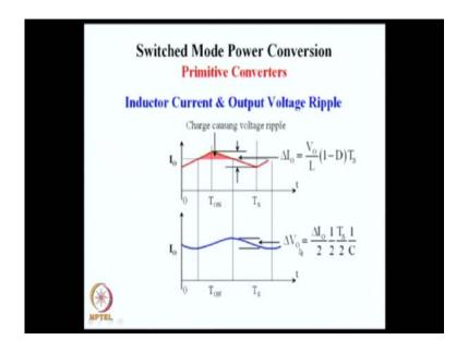
And we can write the delta V naught to be delta I naught by 2 is the height of this triangle and 1 half is for the area of the triangle. And the duration from here to here is what you see here, the duration from here to here is T S by 2 and this entire charge divided by C is delta V naught.
