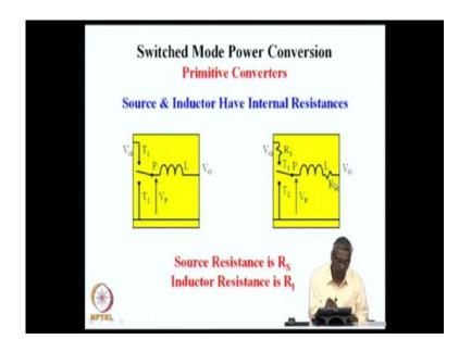
The source can have a resistor as shown here R S and the inductor can have similarly resistance of the winding R L. So, these quantities also give rise to some difference in the voltage transfer ratio. Because these are series non-idealities, they do not affect the current transfer ratio, current transfer ratio will continue to be as before but, let us look at the voltage transfer ratio.
