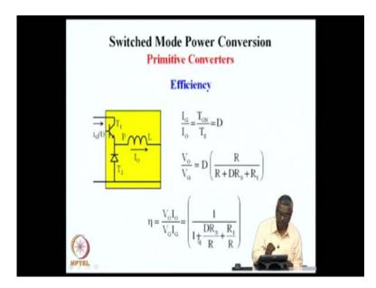
And the consequence of that is the efficiency of this converter is the same as the correction factor in the voltage conversion ratio 1 by 1 plus this R S into D by R plus R L by R. These ratios are small numbers so, in the denominator you will have 1 by 1 plus a
