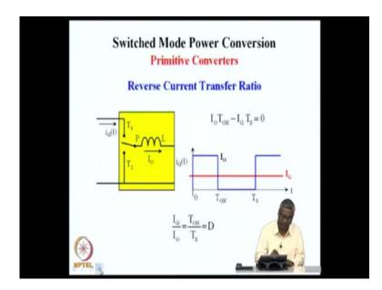
And this can be obtained by simply averaging in the current way form i G of t. What I have shown here for one cycle, the average current of i G of t is given by the red line I G. This i G of t when the switch is ON, it is the same as I naught the current is flowing
