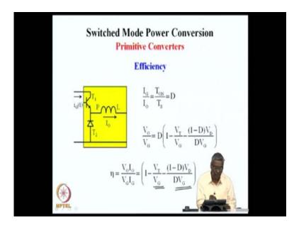
The interesting part is that, now the product of the voltage conversion ratio and current conversion ratio in the ideal converter was 1 which was the efficiency of the converter. In the non ideal converter, I naught by I G is 1 by D V naught by V G is D multiplied by
