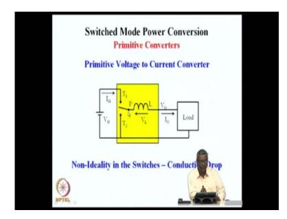
The other non-ideality in the converter is that the switch T 1 P and T 2 P do not have 0 voltage across them. When current is flowing through the switch T 1 to P, there is a small voltage drop across the switch and similarly, when the current is flowing from T 2 to P there is a voltage drop across the switch. This depends on the type of switch that we use.
