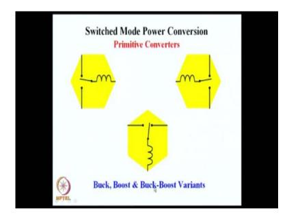
The switch and inductor, what we had analyzed up to now but, inductor at the front and switch at the back feeding to the load is the next configuration. Switch, inductor in the middle and switch connected both to the input and the output is the third configuration. Normally, these three circuits are known as buck converter, the boost converter, the buck boost converter in the power converter topologies or in the power converter terminologies.
