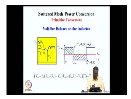
Now, the voltage across the inductor is now the pole voltage minus the output voltage V naught V naught is shown here by the red line. But, the pole voltage now consists of
