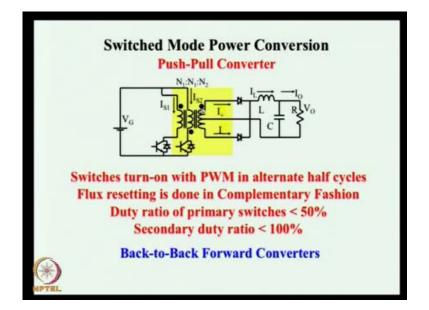
Again for push pull, push pull converter is another derived version of the forward converter or the buck converter the push pull converter is then leads to the half bridge converter, which again other derived version of the forward converter which is another derived version of a buck converter.
