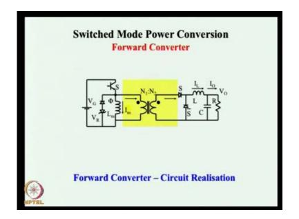
You also have other topics other topologies of the converters the forward converter where in the output side the is filtered, so the switching the EMI and EMC at the output side will be reduced, much reduced switching component or switching ripple on the output will be smaller. Also have isolation galvanic isolation between output and the input, so this is one type of topology. Many derivatives out of rate, which we will be dealing with forward converter the push pull converter.
