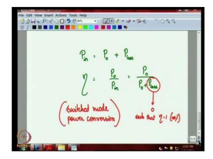
So, the efficiency is P naught by P in or P naught by P naught plus the loss component of the power the whole focus here is to see that this goes towards 0, such that efficiency is 1 or 100 percent in terms of percentage, so to meet the loss 0. The concept of switched mode power conversion is employed the switch mode power conversion basically uses the following concept.
