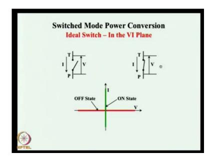
The power semi conductor switches and have a look at what is an ideal switch and do understand about the idealness of the switch and ideal nature of the switch, the requirement that we want it is done with the help of the I V characteristic. This is call the static characteristic, you see here during the off state the switch should be able to with stand voltage both positive are negative and during the on state when the voltage a crosses the switches is 0.
