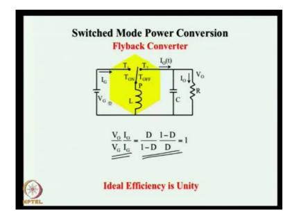
The buck boost converter also called as the fly back converter is a very popular converter which we will discuss much later many converters are derived from this topology. Fly back converter isolated fly back converter is one such and it has a pretty good efficiency to, so this is one of the topics at will be discussed.
