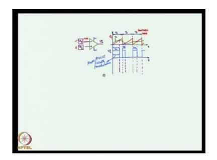
This will be followed by a discussion, I want about discussion on the pulse with modulation. How we obtain the pulse with modulated wave form which will actually be the basics pulses are the gate or the dry pulses, which will turn on the switch turn off the switch the information signal, which needs to be given to them. How do we generate this? How do we go about integrating it along with the controller to give the specific a gate pulse to the various power semi conductor switches?
