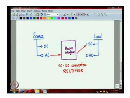
Now, let us take the option. You have an AC and you get out a DC you have an AC input may be from a 230 volts apply grids apply and the output of 5 volts or 15 volts DC supplying to a DC loads, which case you have an AC to DC converter more popularly called as the rectifier. Finally, you have the other possibility of giving an AC input and getting an AC output.
