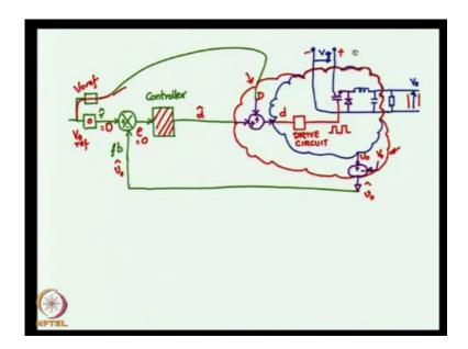
Once we have attained the magnetic module the mathematical model of the DC DC converter, we shall go on to discuss the controller structure diagram, the controller block diagram and how we go about designing the controller for a given switch mode converter system.
