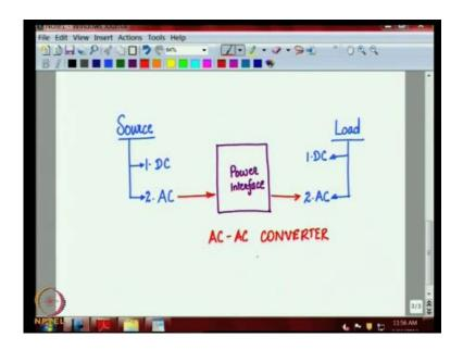
So, you have AC to AC converter, so these are the 4 meter categories of converter that you can, we search. You can see and we will be focusing mainly on DC to DC, DC DC converter only one among the four.
