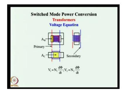
We would also initially we will talk an inductors and later on for the down in the course we will also talk on the transformers and how we would use this transformers and switch mode converters high frequency transformers in a way which will which will give additional degrees of freedom in making the input and output more compactable. They also will be based on the paradise loss V is equal to N by N d pi by d t the fundamental paradise a principles. (Refer Slide Time: 31:06)
