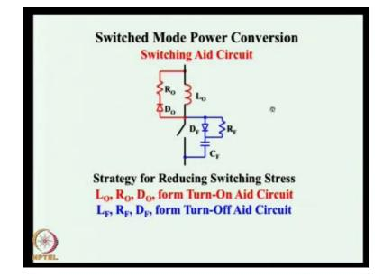
Then while discussing on the switch is in order to address the issue of switching transitions turn on and turn off the stress on the devices maximum during the turn on and turn off, because we see that there is loss during that time. Not only that there are the electrical stresses during turn off the voltage stress across the switch. If there is inductor present the there will be a huge voltage kick which can stress the device.
