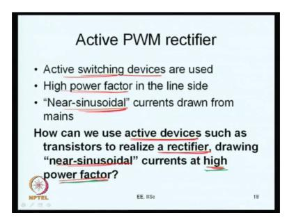
So, what do you do an active PWM rectifier uses active switching devices such as transistors now.
