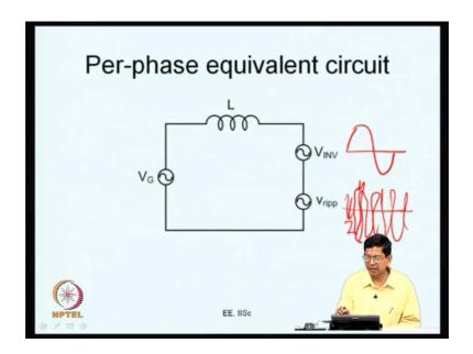
So, it can be either single phase or three-phase if you even if you look at three-phase the per phase is equivalent circuit is something like this what you do is you have the grid voltage this is the per phase grid voltage and this is the per phase inductance now and if you look at the per phase voltage of the inverter it can be decided into 2 one is the sinusoidal component there is a sinusoidal component.
