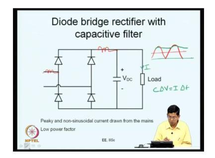
So, now let us say you want rectification the best known rectifier is a diode bridge rectifier and in mostly in power supply applications you will have a capacitance on this side why. Let us say if we have a diode bridge rectifier if you use a resistive load this would be the output voltage waveform will be what is called as a rectified sign now.
