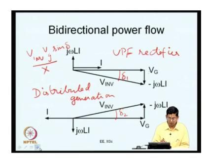
So, now what I am going to say is you are you also have bidirectional power flow; here you can also have bidirectional power, it is not necessary that the current is drawn at unity power factor this is what we saw let us say power is available on the DC side and needs to be pumped back into the mains now which is what you will have. Let us say you
