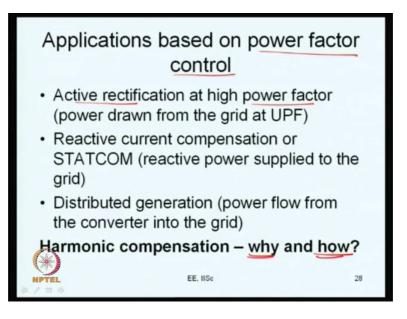
So, from whatever we saw now it is possible for you to you know control the power factor at which current is being drawn now that power factor can be unity that can be are very close to unity the phase difference can be very minimal between the current drawn
