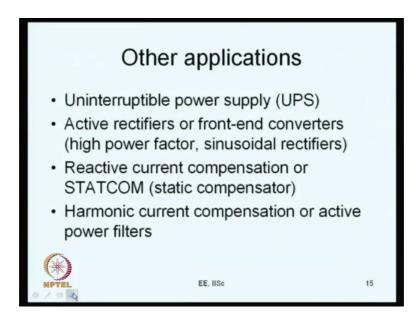
So, there are other applications as we mentioned one is an uninterruptible power supply what do you do this here you have a battery bank essentially when there is no power supply available in the mains the energy stored in the battery bank is what you used to supply the AC load now. So, you use an inverter. So, battery bank whatever you know you through an inverter you feed AC loads there is the output frequency is always 50 hertz or so.
