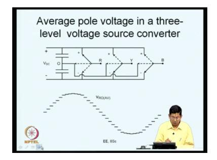
Instead of a 2 level inverter if you take a 3 level inverter and once again VRO average is typically modulated in a sinusoidal fashion, but as I mentioned the way a particular average voltage is realized its different within a switching interval the instantaneous error voltage is lower now that is what results in a better quality waveform here.
