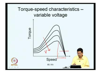
See if with a voltage source inverter you are capable of varying the amplitude and you know applying a variable amplitude on your motor. So, as V decreases your torque speed characteristic reduces changes like this for a higher V the torque peak torque is high for a lower V the peak torque is low. So, the characteristics roughly look like this now.
