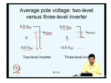
How is the average pole voltage controlled you know this is how more about how an average pole voltage is was realized as I just mentioned in a 2 level converter you apply plus 0.5 VDC for certain amount of time and minus 0.5 VDC for remaining amount of time and you get an average voltage which is indicated as VRO average here now.
