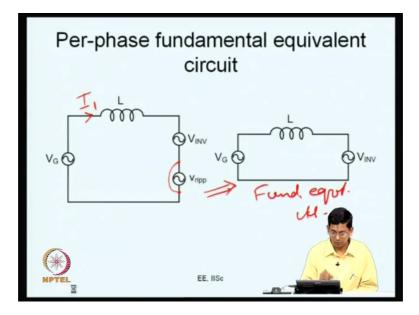
If you want to consider the fundamental equivalent circuit I mean, I want to calculate the fundamental current; the fundamental current I one is not affected by the ripple voltage. So, this is effectively a short here. So, you will be go to this fundamental equivalent
