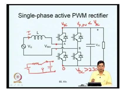
So, you use a voltage source inverter if you have voltage source inverter which has a particular value of V DC which is now steady let us presume that you have an inverter was DC bus voltage is charged now.
