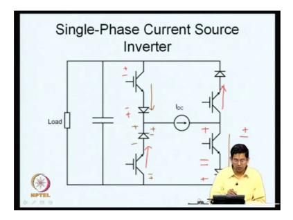
So, you can say if the current is flowing in this direction as it is you will have if these two devices are current flows in this direction and these blocks a potential which can be of either polarity a potential of this polarity is block whether diode and the potential of opposite polarity could be block by the transistor. And therefore, you have a bidirectional voltage blocking capability here.
