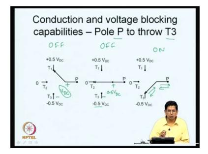
Now, let us look at the next one let us look at the conduction in voltage blocking capability is between the pole P and throw T 3. So, what we are looking as pole P and pole T 3 this is now off state again pole P and throw T 3 it is now in the off state whereas, this is the on state in the on state you know. So, there is always anyway current keeps flowing through the pole and in the on state it flows through T 3 between P and T 3 you need a bidirectional current carrying capability.
