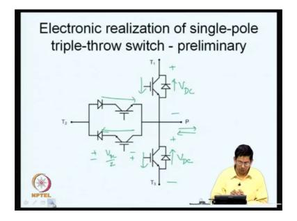
So, all the switches are capable of bidirectional current conduction because through pole P the current conduction can be in both the direction. You can see that all the switches can conduct in both the directions this can conduct this way this can conduct. This way this transistor like this this diode like this can conduct then this direction this can conduct an opposite direction.
