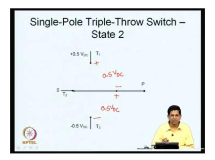
Let us look at state 2 this is state 2 here as we can see P is connected to the throw T two. So, between P and T 1 the devices are off. Similarly between P and T 3 the devices are off. So, between P and T 1 the devices together are blocking a potential where T 1 is positive with respect to P because T 1 is connected to plus 0.5 VDC P is connected to T 2 this is connected to 0 and the potential between these two is 0.5 VDC.
