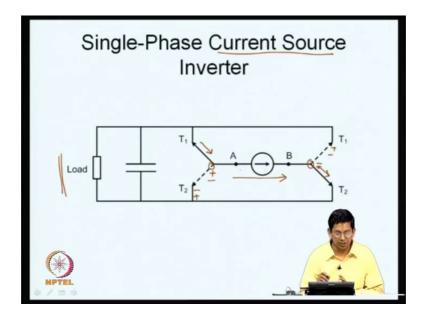
Now, let us say this is the single-phase current source inverter you can see that structurally it is quite similar to a single-phase voltage source inverter what I mean that one with only one difference in in a single-phase voltage source inverter you had a load connected between these terminals A and B and you had supply connected between these two terminals.
