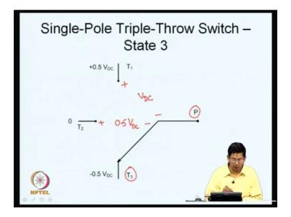
Once again we go to state 3 the pole is connected to the bottom throw T 3 and between P and T 1; T 1 is positive P is negative and the potential differences VDC. So, these switches are in the off condition and they blocking a potential equal to VDC. And similarly the devices that come between P and T 2 block a potential which is equal to 0.5 VDC here as indicated here. So, this is what you have now
