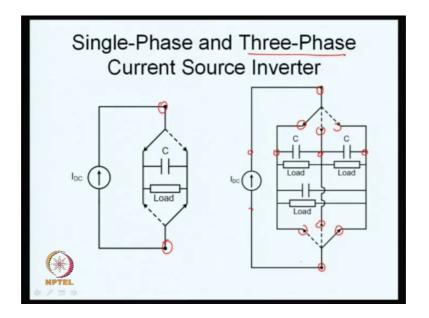
So, I have just drawn a single-phase current source inverter using generic switch now.
