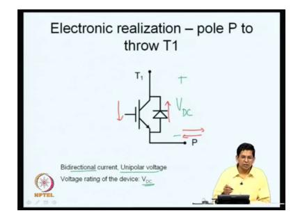
So, how do we realizes electronically this is quite similar to what we saw in a voltage source inverter? So, the current could be flowing in either direction and therefore, we
