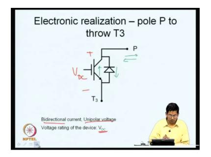
So, this is what we made P quite similar to what we got before if does conducting these can conducting in these two directions if it is blocking it can block a potential like this. So, it is bidirectional current and unipolar voltage and the voltage rating required is VDC.
