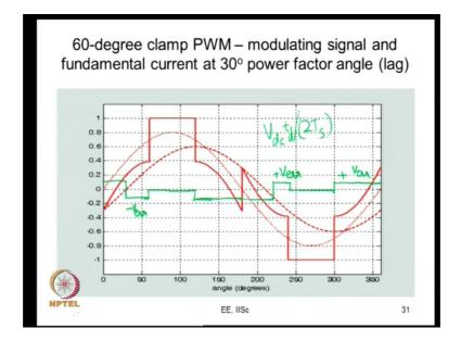
So, let us now look at the next example the same 30 degree and 60 degree clamp PWM, but at 30 degree power factor angle now; so, let me do this error voltage business. So, what is the error voltage here? First consider 30 degrees; so, what is the direction of current? The direction of current is negative up to this point and therefore, my error voltage will be positive.
