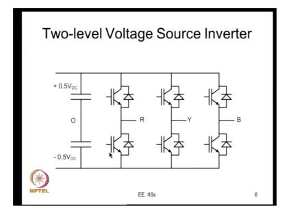
So, now we are talking of the dead time effect in a voltage source inverter. So, first quick look at the voltage source inverter; three different legs single pole double throw switch. The switches are supposed to be switching in a complementary fashion and that is where we have a difficulty now. The gating signal for the top and the bottom cannot exactly be complementary, the rising edges of both of them have to be delayed.
