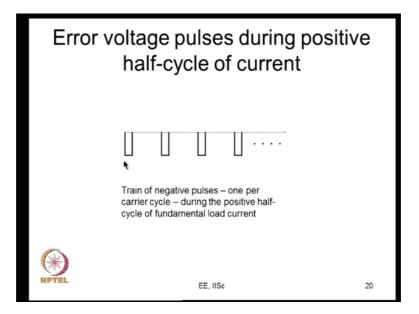
And therefore, you get like this; therefore, you get a train of negative pulses during the positive half cycle of current. So, you will see one error voltage pulse in every carrier cycle.
