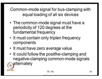
And that is what has been discussed here. So, we have a triplen frequency waveform common mode component added to that and we make sure that all the 6 devices get loaded equally that is; the common mode component will make sure is of periodicity 120 degree, it contains only triplen frequency components, it does not contain any DC component we make sure and we do this.
