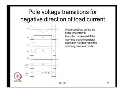
So, this is something which is given for the other direction of current, but the philosophy is same that is during the dead time, it is a diode that conducts. The transition is delayed if the incoming device is transistor; the transition is not delayed if the incoming devices are diode alright.
