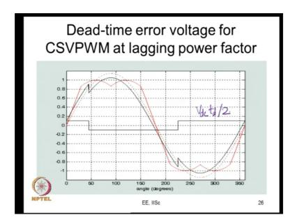
So, this is again we have given the; conventional space vector PWM and this is how the dead time error voltage is.
