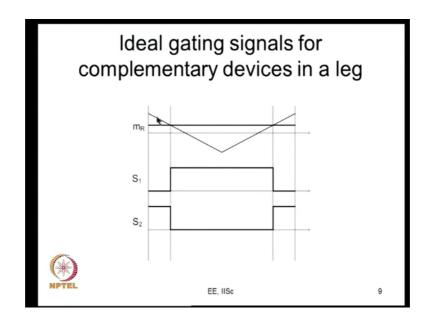
So, normally what you do? You do a comparison; we are now looking at just one carrier cycle. If this is your modulation signal for R phase you compare the output is here; the inverted output or the complementary of that is here. So, this is fed to the top device, this is fed to the bottom device; are supposed to be fed to the top device and supposed to be fed to the bottom device in the R phase like ideally, but the situation is not ideal.
