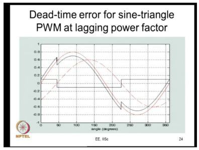
So, these are the error voltage average error in the pole voltage which we saw. So, what we are going to look at is; these are how the variations is, so this is now what I had plotted by hand; here it is shown plotted already. So, this is sinusoidal sine triangle PWM. So, the average pole voltage is expected to be like this, but the average pole voltage actually changes like this.
