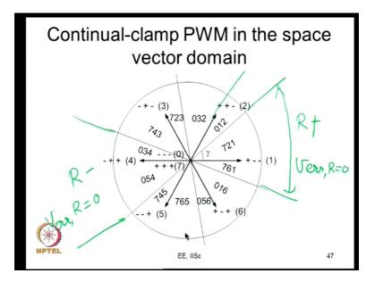
So, now if you look at the continual clamp in the space vector domain, what do you have? This is how you can look at, this is continuous PWM; so, here there is this region over which R phase is clamped to positive bus. And again this is the region over which R phase is clamped to the negative bus, you can see that it is clamped to positive. So, here what you will have is V error for R phase will be 0 in this region.
