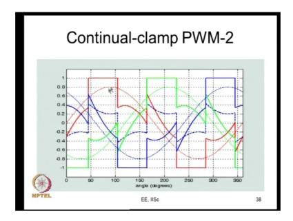
And this is continual clamp where this is; when we saw for switching loss, this is for the lagging power factor load this is to reduce switching loss and leading power factor loads.
