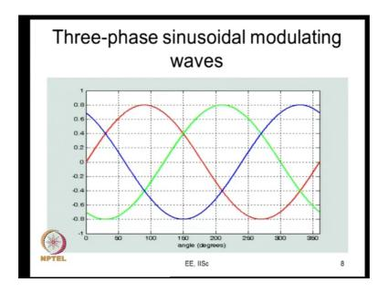
So, once again looking at the best known example of modulation methods like sine triangle PWM; three-phase sinusoidal signals, which correspond to R phase, Y phase and B phase compared against high frequency triangular carrier and you produce the PWM signals. So, the output of this gives the top device and the complementary of that would normally give the bottom device now, there is a small difference; after that there is introduction of dead time as we discussed before.
