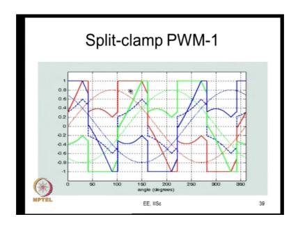
This is split clamp PWM which is good for from the point of view of switching loss, it is good for a loads having power factor angle between 60 to 90 degree.
