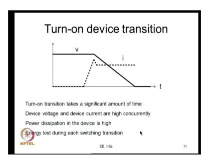
Because the devices are not ideal you need to do something that is introduced dead time. So, what is the non ideality that is affecting us? The finiteness of the transition time, the transition times are not 0, they are significant it takes significant amount of time for the device to turn on.
