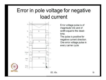
The difference between the two will be V dc, so you will get a; for the so called negative direction of load current, your error voltage pulse is positive.
