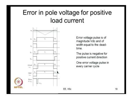
So, because of these rules what happens; whenever your positive so called positive direction load current, the actual pole voltage and ideal pole voltage are like that and you get a negative voltage pulse, there is an error voltage pulse which is a negative voltage
