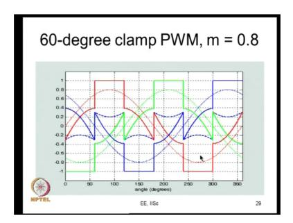
We apply range of PWM methods, so this is the so called 60 degree clamp PWM or sometime called DBWM 1, where a phase is clamped at the middle 60 degrees everywhere now.
