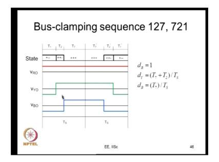
So, the switching sequence is 0, 1, 2, 2, 1, 0 and switching sequence is 1, 2, 7, 7, 2, 1.
