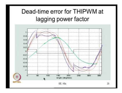
So, this picture shows the fundamental sinusoid; this is the fundamental voltage that you will get. And this is the average pole voltage; the average pole voltage contains several of the harmonic I mean the triplen frequency components. These triplen frequency components will vanish, they are in the average pole voltage they will vanish in the line to line voltage and the load applied voltage.
