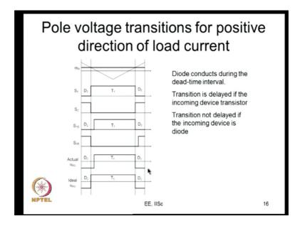
So, now this is where you go your taking a relook at the actual average pole voltage and the ideal average pole voltage now. So, like the diode conducts; so, the diode is conducting here the diode continuous to conduct during the dead time whereas, ideally it should have switched here. So, if there were no dead time between the top and bottom; so it switches here. So, it is here now again, but here what happens the incoming devices are diode.
