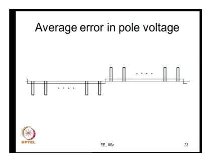
So, which is what is shown in the next slide; so, this is an important information for us and this square wave; gives a measure of how much damage is caused by dead time or how much is the; I mean the fundamental and the low frequency components which have been introduced on account of dead time, at the inverter output. So, this is the reason I drew this before when I did the sinusoidal current, this is what I did. So, this was all that; I have said now were the basis by which I did this now.
