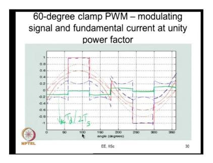
In other regions R phase has an error how much will that error be? It will be the same thing as before. It will be V dc multiplied by t d upon 2 T S and the direction or the polarity of the error voltage will depend upon the direction of current. So, now let us take one case what is this? 60 degree clamp PWM again. Here we had all the three modulating signals before, it is easier if we look at just one modulating signal that is the R phase modulating signal.
