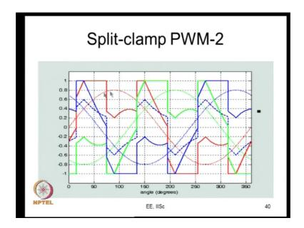
And this is for 90 degree lead; it is I mean this is peak clamp 2, here the sum of these two clamping durations anyway add to 60 degree.
