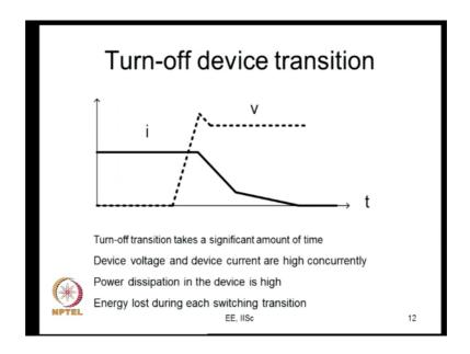
So, R it is better to look at the turning off device because you want that device to be turned off first before the incoming device is turned on. So, what you would do is, so you would have turned off somewhere here and the after certain t d off, off time delay time you will see that the voltage is rising. And after that you see that the current is falling; may be first initially falling sharply and then falling more gradually.
