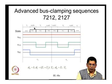
Here what are you doing 7 2 12 so 2 is being applied for 0.5 T 2 times each so these are advanced bus clamping PWM sequences R phase is clamped B switches once, but Y switch is twice as I told you this will be advantageous if the energy that you have saved by not switching R phase is greater than the energy that you are losing by switching the Y phase or in other words if the R phase current is greater Y phase current this is an advantageous otherwise this is a disadvantageous.
