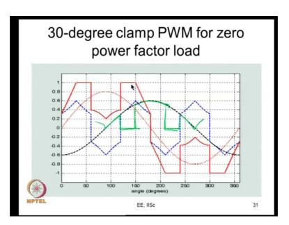
So, I have found it more clearly here. So this is for example, is the R phase modulating signal for 30 degree clamp PWM it is R phase modulating signal this is the common mode component for the 30 degree clamp PWM you add that then you get your R phase signal like this.
