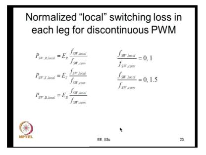
So, what happens in bus clamping PWM if you look at R phase you will have an R phase switching energy loss which normalized R phase switching energy loss as we derived and discussed before this is simply proportional to i R.
