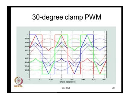
For the same example, let us say you take 30 degree clamp PWM; now what this 30 degree clamp PWM does is, it clamps here like from 120 to 150 degree the R phase is clamped. So, it is 0 power factor load so you will see that here it is 0 crossing at 120 degrees it will be 0.5 times the peak value, here it will be 0.866 times the peak value, so it will actually be clamping the current when the current is between 0.5 times it is peak and 0.866 times it is peak.
