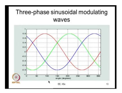
So, let us start off with our sine triangle PWM three-phase sinusoidal signals are there. So, this is for R phase, Y phase and B phase and you compare them with the high frequency triangular carrier and feed them so to the inverter.
