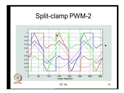
The other example is this is 50 and this can be 10 we call this split clamp PWM 2, so this continual clamp PWM and split clamp PWM together represent the complete range of bus clamping PWM methods except 120 degree clamp. So, these are the PWM methods which can ensure that all the 6 devices the converter operates in a balanced fashion so this actually summarises everything.
