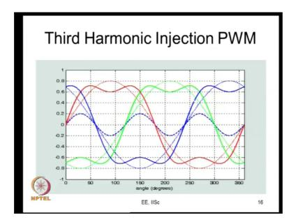
So, when this also this is an example of a third harmonic injection, so like another continuous PWM method why do you say continuous PWM method you look at the modulating signal, the modulating signals are continuous function of time or the fundamental angle so and all the phases are switching all three-phase three-phases are switching there is no phase which is clamped here alright, so the losses are same now.
