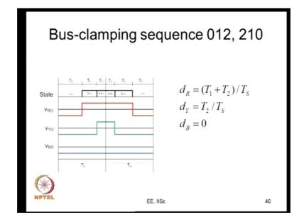
If it is bus clamping PWM method what do you do? You apply let us only 0 for the entire duration T z or you know 0, 1, 2, 2, 1, 0 so this is one way of doing bus clamping PWM.
