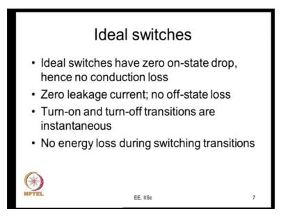
So, as we said the ideal switches will not have any forward drop and therefore, no conduction loss there is 0 leakages, current. Therefore no off state loss, and they turn on or turn off in an instantaneous fashion there is no energy loss during switching transitions that is about the ideal switches.
