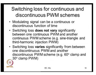
Now, just to summarize or whatever or recap can be modulating signal can be continuous or discontinuous and the switching loss does not vary significantly from one continuous to another continuous PWM scheme, whereas it very significantly from one discontinuous PWM to another as we saw some examples yesterday and so now ours whatever we want to do like designing PWM schemes. Obviously, these are not going to be continuous PWM schemes.
