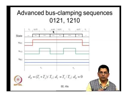
Similar exercise can be carried out for all the other sequences. iIf this is advanced bus clamping PWM you are just doing 0 1 2 1, 1 is being applied 2 times for 0.5 T 1 seconds each.
