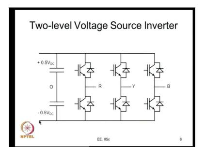
Now, let us get started this is the three phase inverter this is three-phase load which is not known I mean this is not shown here in the figure there is this dc side. And you know there are losses in these devices both the transistor and IGBT etcetera we have this now and there are conduction and there are also switching losses the present focus is really on the switching loss ok.
