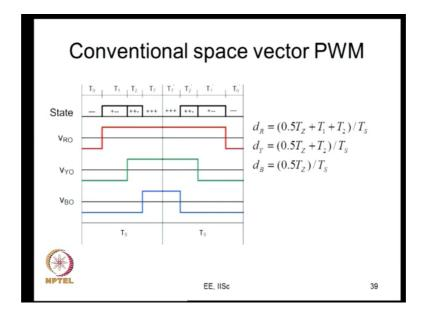
So, we are going to apply the vector states like 0, 1, 2, 7, 2, 7, 2, 1, 0 like this when you a space vector PWM the active vector is are applied for a T 1, T 2 seconds, the null vector is applied for T z by 2 and T z by 2 here if it is conventional space vector or it can be
