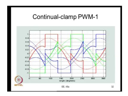
Now we will generalize this now this is continuous clamp PWM. So, what you do you can clamp a phase for 60 degrees continuously. So, to a particular bus here again the same phase is clamped to the other bus for 60 degrees continually. Therefore you call it continual clamp PWM. So, this is oriented towards lagging power factor loads so I am calling it as Continual-clamp PWM-1.
