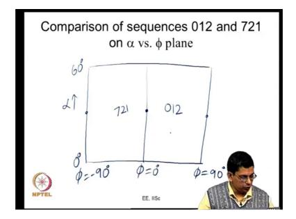
So, you can actually represent it like this what you are trying to do is let us say you can consider a particular box. Now here this is the power factor angle phi is equal to 0 degree, phi is equal to 90 degree, phi is equal to minus 90 degree so one side it is leading, the other side it is lagging.
