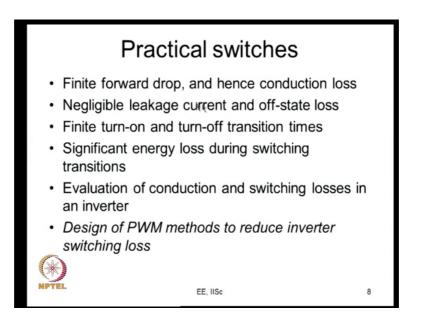
What about the practical switches? They have finite forward drop therefore there is certain amount of conduction loss and there is negligible leakage current and therefore, the off state loss is also negligible we do not have to worry about that.
