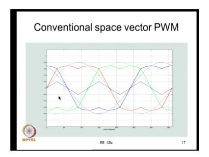
So, this is true about conventional space vector PWM also. So, in conventional space vector PWM this is your fundamental sinusoidal modulating signal. And this would be the kind of common mode added and you would get a modulating signal which is like this, it is also here also the switching loss is same as we discussed before.
