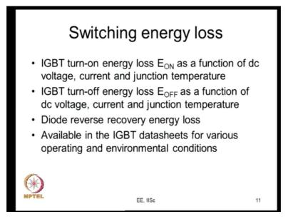
So, there is this energy loss turn on energy loss E ON, this turn off energy loss E OFF, these are available as functions of dc voltage, current and junction temperature these are normally they are available in the data sheets. Similarly the diode has what is called as reverse recovery energy loss so there is a reverse recovery process, there is some energy losses that.
