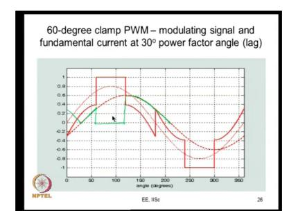
There is another particular case we are taking now so in this case if you see a phase is getting clamped. But where is the current? The current is actually little lower and here so here the current is high it might have been advantageous if the phase could have been clamped here but the 60 degree clamp PWM is not really clamping like that.
