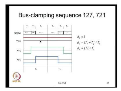
This is the other way of doing bus clamping PWM, you apply only the 0 state 7 the entire T z you apply this 0 state 7 so 0 never gets separate in this case R phase gets clamped in the previous case the B phase was getting clamped to the negative bus here R phase is
