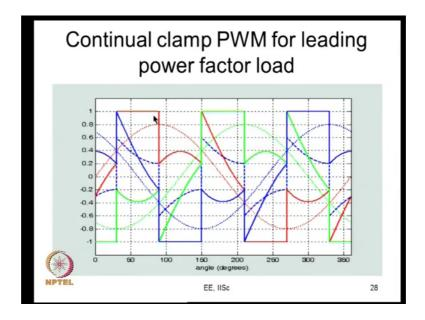
If you are talking of 30 degree leading power factor case sometimes load could be leading power factor in that case this is helpful. So, if the load current is 30 degree leading power factor then this would actually result in the best possible reduction that is possible with this now. So, we are looking at everything in terms of the modulating signals right now after while we will go into the space vector domain and we will do it a little differently.
