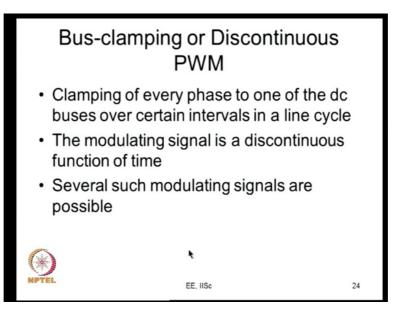
So now in bus clamping what happens? Every phase is clamped to one of the dc buses over certain intervals in a line cycle. And that is typically the phases clamped to the positive dc bus for 60 degrees and to the negative dc in another 60 degrees. So, the modulating signal is a discontinuous function of time. Then you have several such modulating signals are possible, that is what we have seen before.
