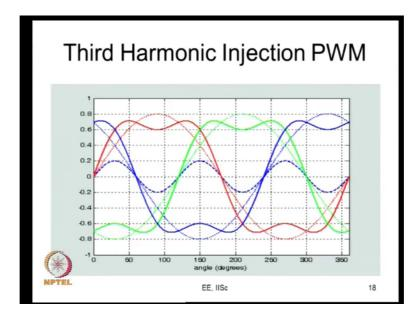
So now you go with PWM method. By PWM method I said that this procedure is common for anything now. So, it is not just sin triangle PWM, what I have done is on this modulating signal I have added common mode for all the three-phase modulating signals. So, your R phase signal looks like this. So, the common mode signal is a third harmonic signal. So, that is why I call this is third harmonic injection PWM we have seen this before.
