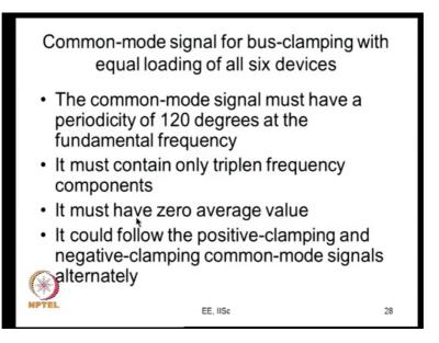
So, one simple exam; so if those are many variations, what we try to do is the common mode signal should have periodicity of 120 degrees; it must contain only triplen frequency components. So, it will follow the positive common mode for 60 degree, and the negative common mode for 60 degree. And it will also have a 0-average value.
