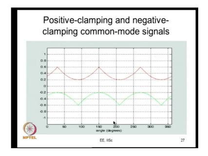
So, when you are adding this common mode, we have to make sure that the top and the bottom devices are balanced, and the losses in all the 3 are balanced. So, if you want to make sure that top and bottom are balanced, what we have is; this is the positive clamping common mode signal. And this is the negative possible common mode signal. You can either follow this or follow that.
