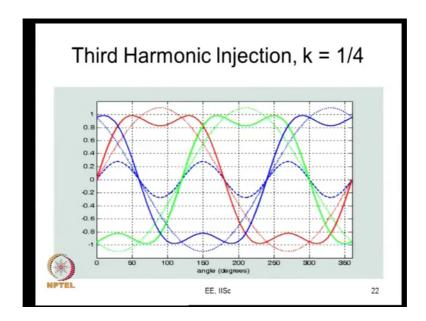
With third harmonic injection, your common mode I mean or the total harmonic distortion is minimum wave form quality is best when you add k equals 1 by 4. That is
