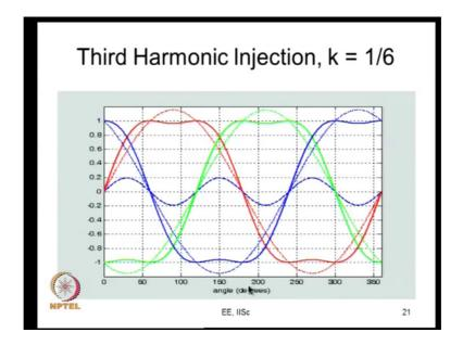
So, this is the 1 by 6 which has been illustrated here. Actually, it is about 2 by root 3 is your sign peak is 2 by root 3 times V peak, and with the common mode added you can see that your modified common mode m R star just touches 1, it does not go beyond 1. So, you are within linear modulation, and you are able to produce this PWM highest dc visualisation.
