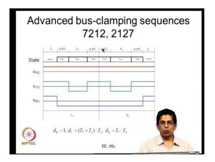
Similarly, if you look at the sequence 7 2 1 2; so here R does not switch at all duty ratio is one, what is a Y phase duty ratio? It is T 7 which is basically T z plus 0.5 T 2 plus another 0.5 T 2 divided by T s. So, it is T 7 plus T 2 by T s, what is duty ratio B phase? It is T 7 divided by T s.
