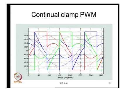
So, this is continual clamp PWM; that is 60-degree clamp is a particular case of this. This is a little more generous. So, what we have no claimed is we have not clamped between 60 to 120, but earlier we had clamped now we are clamping between 30 to 90. And again, here we are clamping it between this 210 to 270. So, this is again here is a different modulating signal, this gives you the duty ratio. You can go by this duty ratio to calculate your D R.
