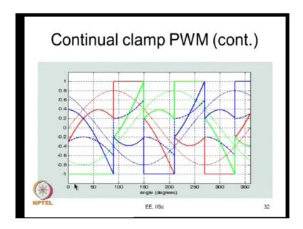
This is another clamping. So, every where once you know the modulating signal, you can find out the duty ratio. How the duty ratio varies as a function of omega t and you can do these calculations.
