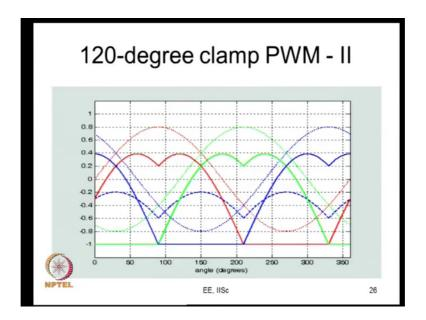
This is the other 120-degree clamp PWM here. What is happened is; you have added this kind of common mode component which is always negative. So, here the bottom device is tend to conduct for longer than the top devices. So, you can see that the bottom duty ratio is always 1. So, you may have more conduction loss in the bottom device than the top device. So, it is unequal.
