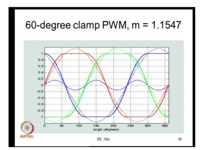
Again, this is again 60 degree clamp it is illustrated for 1 is equal to 1.1547, that is m is equal to 2 by root 3. That is the modulating signal as a peak value 2 by root 3 times the peak of the carrier. So, in this case the modified modulating signal just goes and touches one and stays at one and comes down. If you go little above this, it will go into what is called as over modulation. So, this is the highest possible thing, and again how will you
