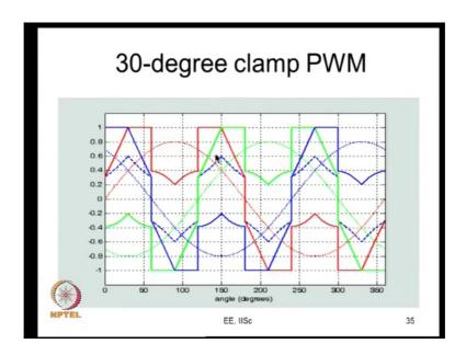
So, this is a split clamp PWM. What happens is that; it is not clamped continuously for 60 degree; it is clamped for some 30 degree here and 30 degree here. And so, we call it 30-degree clamp PWM here. So, here again if you want to calculate the conduction loss, you can see the duty ratios go by this now, ok.
