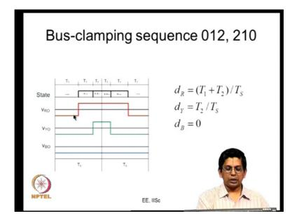
Again, if you looking at the switching sequence from the space vector point of view like this; this is bus clamping sequence 0 1 2 2 1 0 you are using only the 0 state 0. What is the R phase duty ratio? The R phase duty ratio is T 1 plus T 2 by T s. What is the Y phase duty ratio simply T 2 by T s. What is a B phase duty ratio? 0 B phase it is always it is minus B dc by 2 it does not switch at all the top device is never on. So, it is 0.
