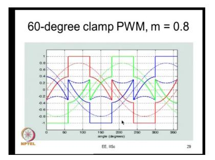
So, if you this is what we would do to come up with most of the popular bus clamping PWM method. This is one popular bus climbing PWM method, which is called 60-degree clamp.
