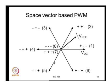
Now, if you want to do the same thing using space vector based PWM. So, of course, for continuous and discontinuous PWM methods, you can construct the method as an equivalent modulating signal and you can do that; that is always fine, but let us anyway look at it in from this point of view also. You have a revolving reference vector. You are sampling it in once and every sub cycle time.
