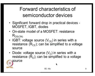
So, you have this, what are the go by individual devices, there is MOSFET there is IGBT there is diode. So, if the MOSFET is conducting, what is the relationship between the voltage across the MOSFET and the current through the MOSFET? That is what is called as forward characteristics; relationship between the forward voltage and the forward current that is when the device is conducting, what is the voltage drop? We see the current through the device.
