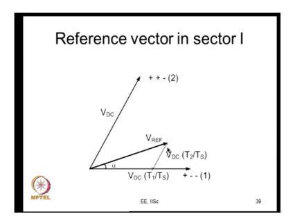
And then you are going to apply this vector for a T 1 seconds, and this for T 2 seconds, and the null vector for T z seconds. To realise this vector in an average sense, we know this.
