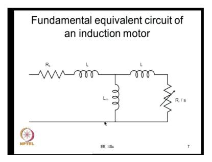
So, the fundamental component gets applied you know, on the motor, it is the one that produces the torque essentially, the steady torque. So, the current produce you know is can be calculated by this. This is the fundamental equivalent circuit. You want analyze the effect of the fundamental voltage on the motor, you can use this equivalent circuit now.
