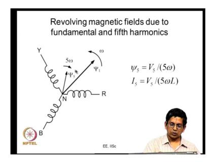
So, this produces one. What is the frequency? So, let us call it psi 5, and this psi 5 would be V 5 by 5 omega. So, this is a revolving magnetic field, but it revolves at a frequency 5 omega, and in the opposite direction compare to omega. So, the relative speed between the fundamental magnetic field and the fifth harmonic magnetic field is 6 times the fundamental frequency. And this is why it leads to what is called as 6th harmonic torque.
