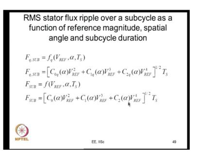
So, you will actually get this as one function. This is the q axis ripple, you will get it as some function V ref alpha Ts. And you will get the total stator flux ripple also some function of V ref alpha and Ts. And the nature of the function is actually shown.
