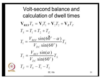
And this for t 2 seconds, and t at the null vector for the remaining once, and how are they calculated? This is what is volt second balance. This is a reference volt second, this is the applied volt second, and they are equal. And the sub cycle time is equal to the active vector time 1, active vector time active vector 2 times and you know the null vector time.
