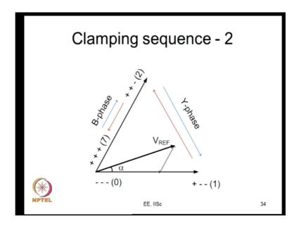
There can be another clamping sequence. For example, you can avoid this 0 stat 0 fully; let us say you start from your active vector 1, apply this for t 1 seconds. Switch your Y phase and move here. Apply this vector for t 2 seconds, then switch your B phase and move here, stay here for t z seconds. Your sub cycle is complete, your produces this reference vector. In the next sub cycle, you will have to produce another reference vector, which will be close to this; on different bicycle angle.
