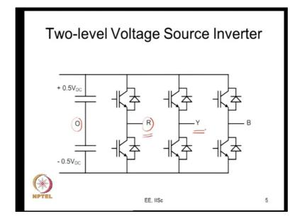
So, it is a usual three-phase voltage source inverter, and R Y B are the load terminals you have connected the motor here. And this is your dc bus, and this is dc bus midpoint. This dc bus midpoint is convenient for measurement of voltage at R Y and B. So, you call it V R O, I mean (Refer Time: 06:04) V R O is something we called as pole voltage. V Y O is Y phase pole voltage, and V B O, we call this as B phase pole voltage. And you subtract V R O and V Y O, you get V R Y, and so on so forth.
