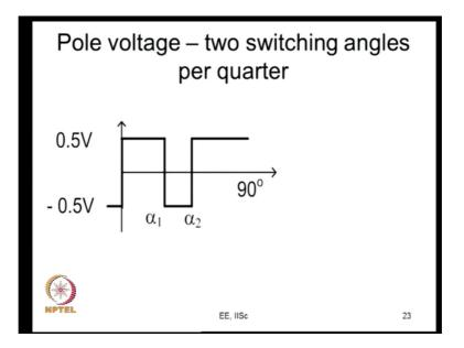
So, just as we could eliminate harmonic voltages. So, for the elimination of harmonics voltages, we had considered the simplest a case where we have 2 switching angles per quarter.
