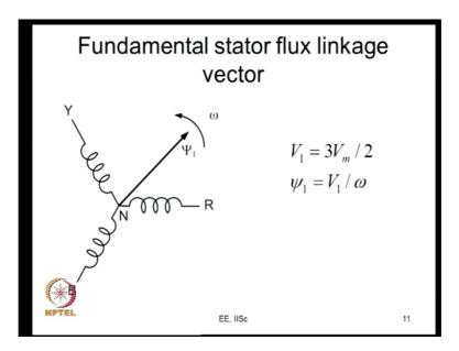
So, the fundamental one produces the fundamental flux. So, you have the three-phase voltages, they are transformed into space vector. You have a vector of magnitude V 1 and you could think of a corresponding vector, that is a stator flux leakage vector. The magnitude of the stator flux leakage vector would be V 1 upon omega. So, and this is a vector which revolves like this, this is produces a fundamental magnetic field. Let us move on to the next.
