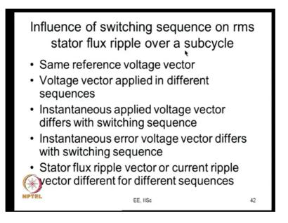
So now what happens? With switching sequence, you may generate the same reference voltage vector, but the voltage vector is applied in different sequence. Therefore, the error that is the applied vector minus reference vector is different. So, they apply instantaneous applied voltage vector differs with switching sequence. Therefore, the instantaneous error voltage vector differs with switching sequence.
