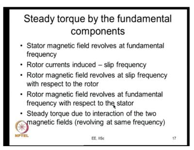
So, what happen because of that? So, the stator magnetic field revolves at fundamental frequency. These we are trying to look at the fundamental component alone, or simply the sinusoidal operation. So, the stator magnetic field produces a revolves at the fundamental frequency, the rotor currents there is some EMF induced the rotor. So, that is at slip frequency. So, this MMF wave it goes past the rotor at slip frequency.
