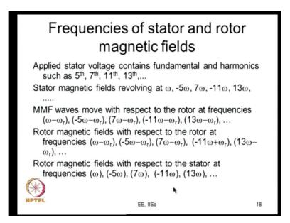
So, when you apply fifth harmonic voltage, it produces something revolving. That is at 5 omega, since it is in the opposite direction we make it minus 5 omega. So, the rotor is anyway rotating at omega r therefore, you know it sees an MMF wave moves pass the rotor at this frequency, minus 5 omega minus omega r all right. So, frequency you know EMF induced EMF in the rotor of this frequency 5 omega plus omega r. Such you know
