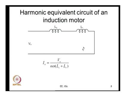
Other than the fundamental there are harmonics, for analysing the harmonic you can use this harmonic equivalent circuit, where this L s and L r are the stator and the rotor
