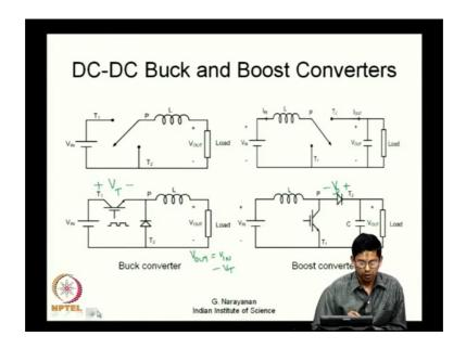
So, we have all of them put together, so essentially DC to DC this buck as well as boost converters have one single pole double throw switch now. And you see that this pole is always in series with the inductance because the inductive current should not be opened and you should always provide a path for the inductive current flow through
