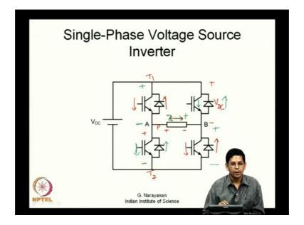
So, you want to come up with a particular set of electronic switches now. What you do? Is you can have a switch like this. So, you can have a bidirectional conduction here, you can have a bidirectional conduction; any direction the load current might be flowing now.
