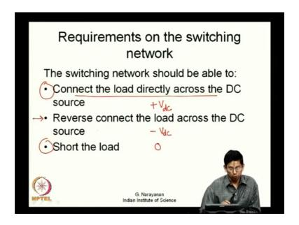
So, the switching network should be capable of connecting the load directly across the DC source; that is you are producing an output equal to plus V. If you call V DC as the input voltage, DC input voltage it should be capable of applying plus V DC between the two output terminals. Again this switching network should be capable of reverse connecting the load across the DC source that is; it should be able to produce apply an output voltage of minus V DC also.
