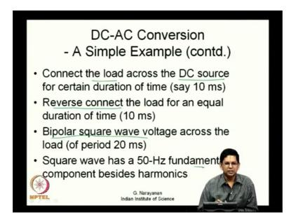
What are we doing here essentially is; we are connecting the load directly across the DC source for some duration of time. And what are we doing? We are reverse connecting the load for certain duration of time. You connect the load for some 10 milliseconds, reverse connect for 10 milliseconds, you connect it for 10 milliseconds and reverse connect you go on doing this way. So, you get some plus V and minus V, plus V and minus V across the load and a square waveform as we saw before.
