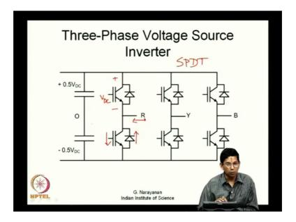
So, it is just same as the same thing that we used earlier, you have a top transistor with an anti parallel diode and a bottom transistor with an anti parallel diode; this will serve the purpose now. So, this for example can conduct in both the directions; the bottom transistor is on, this can conduct; the transistor will conduct in this direction or the diode will conduct in this direction depending on the direction of your load current here, whether it flows this way or that way.
