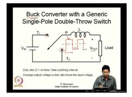
Before looking at DC to AC converters, let us have a quick recapitulation of what we saw about DC to DC converter. Because DC to DC converters are the most fundamental converters and the understanding that we develop with these converters could be
