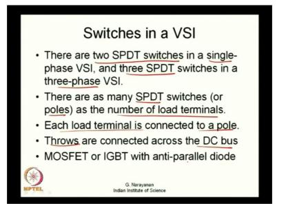
So, some points are made here; how are these switches are connected in a voltage source inverter? Here some observations we are summarizing. There are two single pole double throw switches; in a single-phase inverter. In a three-phase inverter, you have three single pole double throw switches. So, as I mentioned here; there are as many single pole double throw switches or as many poles, as there are load terminals.
