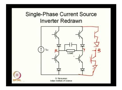
You have one more leg connected like this and this becomes an additional load terminal, you can have capacitance here. And similarly between these two terminals, you can have capacitance connected and load also connected here. So, you can change your single-phase inverter into a three-phase inverter; let me erase these load parts.
