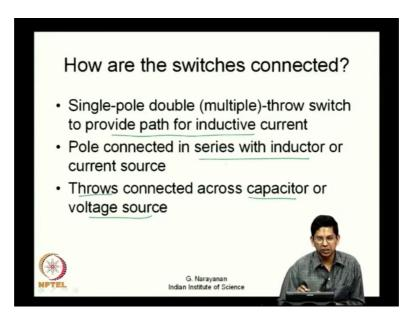
So, here we find certain rules here what do we find about how switches are to be connected; what do we find? We find a single pole double throw switch is used; why is it used? To provide path for inductive current, there is a inductive current and it has to you know be provided with the path, it cannot be opened.
