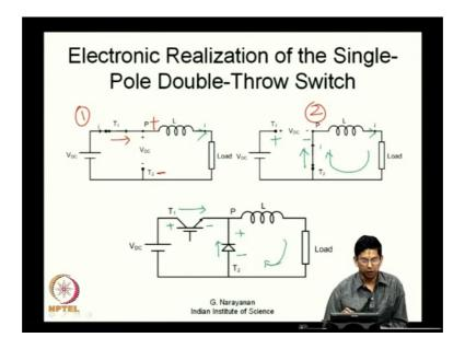
So, we look at the two states of the DC to DC converter, let us call this as state 1 and let us call this as state 2 what happens in state 1 pole is connected to throw 1 and in state 2, this pole is connect to throw 2. In the so called state 1 there is current flowing from throw 1 to pole as indicated in this direction. Then this pole to throw 2 what happens here is, it is blocking certain voltage.
