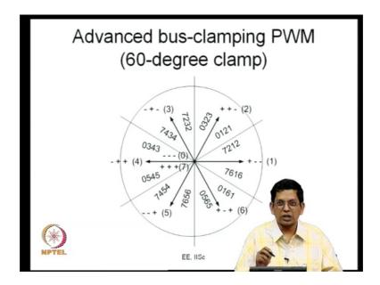
We are now I mean I am taking a quick review of this we are no basically focused and finding out what is going to be the you know DC bus utilization. So, you know going to you know bus clamping to advance bus clamping what you can do is in the so called continual clamp you can replace the 7 to 12 by 0 721 by 7212 or 012 by 0121 and this
