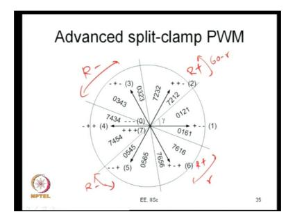
So, let us just look at how the R phase would be the R phases is clamped here to our plus here also it is R plus this is for a duration gamma and this is for a duration 60 minus gamma. The same way you will find R phases clamp in this portions also, but to the negative phase you will find them clamped in these regions also this will be R clamp to the negative bus.
