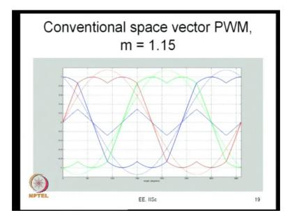
So, as I have also mentioned before as the k is equal to 1 by 6 we can go to 0.577 V DC. And if you go to conventional space vector PWM. So, the third harmonic component there is triple frequency component is. So, this is the sinusoidal component.
