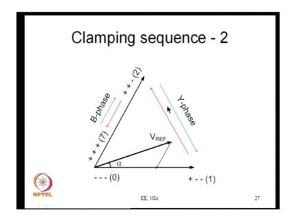
Now, you know alternatively this is skip minus minus minus and so you can use this plus plus plus can be applied for T Z seconds this for T 2 seconds and this for T 1 seconds if you do that you can see B and Y are switching, but R phase is not switching now.
