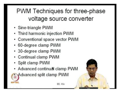
So, a quick list of the PWM techniques that we have looked at in the last couple of modules. So, sine triangle PWM is the most popular PWM method you use three-phase sine waves you compare them against a command triangular carrier and the you produce the PWM signals right.
