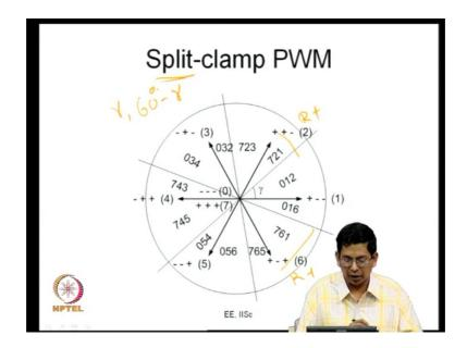
Instead if you go to split clamp PWM as I mentioned before you have the situation where R phases clamp to the positive bus here and R phases clamped to the positive bus in this case. So, these are the durations now. Now you can see that durations are unequal and this duration is gamma and this duration 60 minus gamma they add up to 60 degree. So, the 60 degree continual clamp was split into 2 parts one of gamma and the other one equal to 60 minus gamma and that is what is split clamp PWM.
