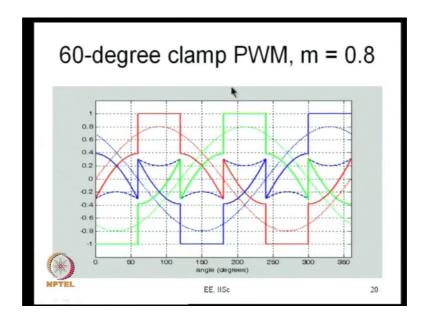
The same way with 60 degree clamp PWM when you want to clamp the middle 60 degree duration, so what you are doing is you are adding a common mode signal as shown by this blue dashed line and the resultant modulating signal is something like what you have shown here right.
