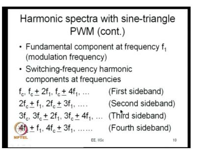
So, there is what you have here is you have the fundamental component frequency f 1 which is a modulation frequency then you have the switching frequency harmonic components now. And the switching frequency components you look at here this around f c you can call them as first sideband and there are components around 2 f c you can call them as second sideband, third sideband, fourth sideband, fifth sideband and all that.
