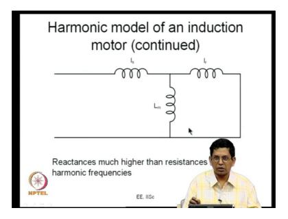
On the first the rotor resistance is low and therefore, you can neglect that and that too at high frequencies the reactance the harmonic frequencies or high frequencies the reactance is much bigger than the rotor resistance. So, you can certainly you can neglect that.
