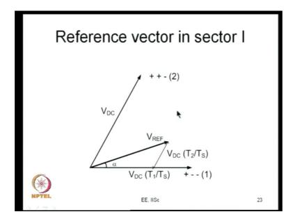
We will apply the vector 1 for some duration T 1 seconds vector 2 for some durations T 2 seconds such that V DC times T 1 by T as in V DC times T 2 by T S simply add up to the required V REF and T 1 plus T 2 is less than the total sub cycle time and the remaining time for you know that is T S minus T 1 minus T 2 for that time we will apply the null vector which is here right.
