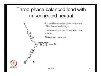
So, you know this is a typical kind of load that we have. You can probably regard this as a stator winding of a machine. So, R is connected to the midpoint of R phase leg why mid phase leg and B is to that midpoint of that leg and N was the load neutral this is not particularly connected anywhere else, but through the R Y and B.
