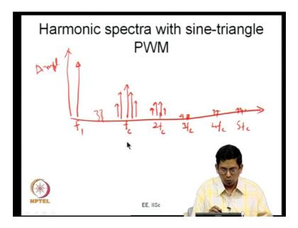
So, I want to look at the harmonic spectrum this is frequency on the horizontal axis and amplitude on the vertical axis. So, what you will certainly have is you will have a fundamental component, you will have a fundamental component let me call this as f 1 this f 1 is same as the modulation frequency.
