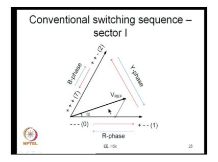
So, you do all this and you look at the switching sequence the calculations are you know we here you calculate T 1 T 2 and T Z and in conventional space vector PWM you use both the 0 states. So, you upload this for it is it by 2 seconds then go here T 1 seconds go here at T 2 seconds and go here for T Z by 2 seconds and then you come back. So, this is what you do in conventional.
