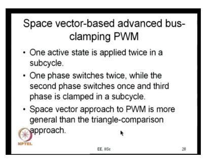
This is about triangle comparison in space later approaches and we just go down and to see space vector based advanced bus clamping PWM, here also you what you have is one active state is applied twice in a sub cycle that is the important difference. In the previous cases all the previous cases you have an active state getting up red only once in
