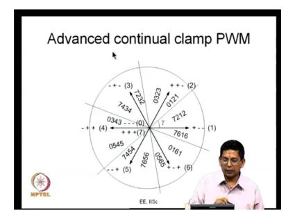
So, now this is advanced continual clamp PWM, this is continual clamp PWM and there is some gamma. Gamma can be anywhere between 0 1 60 degree and instead of 7 to 1 I have written 7212 here, instead of 0 1 2 I have written 0121. So, I will use the sequence of 7 2 1 2 2 1 2 7 it is a trial go on switching that like this and here again I will do 0 one 2 1 0 1 2 1 1 2 and 0 and I will go switch like this.
