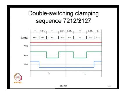
Now, you go here this is double switching sequence 7 2 1 2 this is not 7 2 1 this is 7 2 1 2, you apply 7 for a duration T 7 is equal to T z, then you apply T you apply active vector
