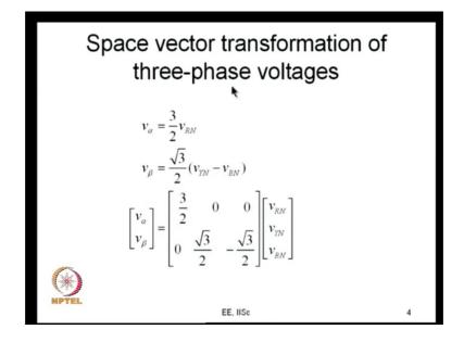
And now here we go back to the space vector transformation of three-phase voltages will quickly look at in what is this transformation, we have known this you know we have been doing this over the last 3 classes. So, v alpha is equal to 3 by 2 times v RN and v beta is root 3 by 2 times v YN minus v BN, this is where space vector transformation right and the same thing has been written in the matrix form here.
