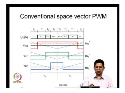
So, this is what is shown in with against time, this is the inverter state up right against time. You have inverter state 0 minus minus minus, you have inverter state plus minus minus, you have inverter state plus plus minus and plus plus plus these are applied for durations T 0, T 1, T 2 and T 7 respectively as shown here now, right.
