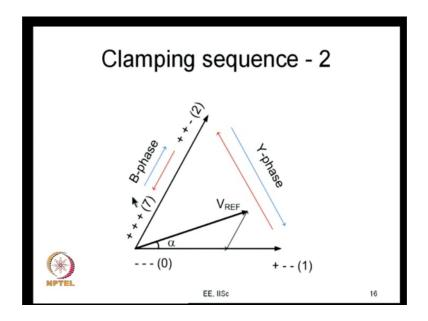
The same way you can skip the zero state minus minus minus totally, and apply only plus plus plus for the entire duration T z; so from plus plus plus you switch B phase you go to plus plus minus and you switch y phase and you go to plus minus minus. On the same way you can go back 1 2 7 7 2 1 1 2 7 7 2 1 and so on excuse me.
