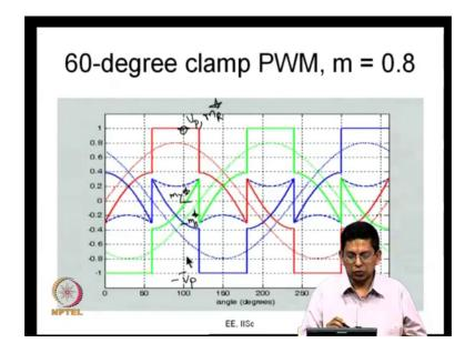
In a in every half cycle we could call it as 60 degree clamp PWM and this is the modulating these are the modulating signals as we saw before.
