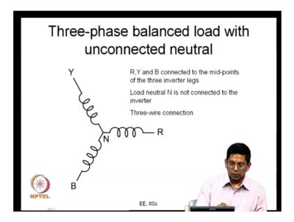
So, know about the regarding the load we have the load R Y and B connected like this and the neutral point N is not electrically connected anywhere else except through the windings to these terminals. So, we are looking at a three-wire connection you know that is how the load is now.
