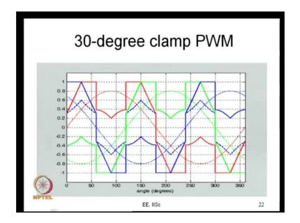
So, here again the a switching frequency is 0, here again the switching frequency is 0 here it would switch at carrier frequency. So, once again you know what you will have is for 60 degrees it is not switching, 30 degree here and 30 degree here and your average switching frequency will be 2 by 3 times fc, you are fc is here carrier frequency right.
