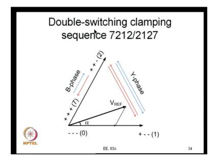
So, this is about 7212 here instead of using 0 I am using 7 and from 7 I go to 2 a stay here for T 2 by 2 seconds, I switch y phase and go one and apply active vector 1 stay here for T 1 seconds and switch back and come here and apply this for the remaining T 2 seconds.
