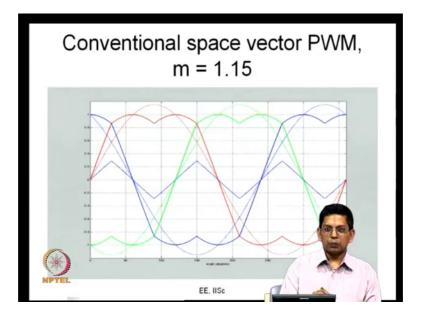
So, this is only to show that you can go a little higher than that, that the modulation you know this is one corresponds to the peak of the carrier do. You see that the signs the peak of the sine wave is 1.15 some 15 percent higher than the peak of the carrier, still what happens? When you add the common mode component, the effective value comes below and the peak value is just touching one.
