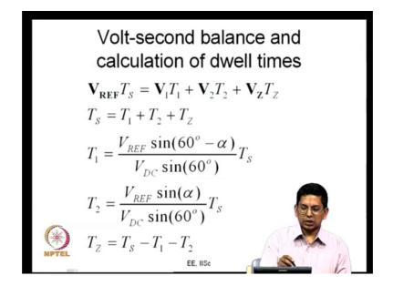
So, that is the equations here, this is the commanded reference vector and this is the applied vector here and the active vector 1 is to be applied for duration T 1, and active vector 2 for T 2 and null vector for T z how do you calculate T 1 T 2 and T z? You get them here, this is T 1 in terms of V REF in alpha T 2 in terms of V REF in alpha and T z that is T s minus T 1 minus T 2, we have seen this in the last 2 3 lectures just having a quick brush throw fall that now.
