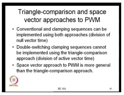
So, I am concluding a few things like this, conventional and clamping sequences many sequences are possible these are possible using both the approaches and division of null vector time is what is essentially done here. Whereas, double switching clamping sequences cannot be implemented using triangle comparison approach, this involve division of active vector time and active vector applied more than twice this is possible only using the space vector approach.
