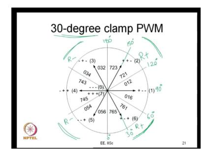
So, this is again you have your 30 degree bus clamping and in this 30 degree bus clamping if you just let us focus just on the R phase alone, you will see that R phase is clamped to the positive bus here and R phase is clamped to the negative bus here. Again you will find that R phase is clamped to the negative I mean positive here negative and here also R phase would be clamped to the negative bus here.
