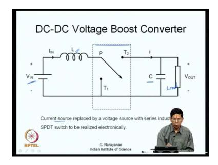
So, what we are doing is, this current source as before we can replace it by a voltage source with a series inductance. As a same single pole double throw switch here and there is a capacitance and load is here this is the load. So, you have what is called as a DC to DC voltage boost converter now.
