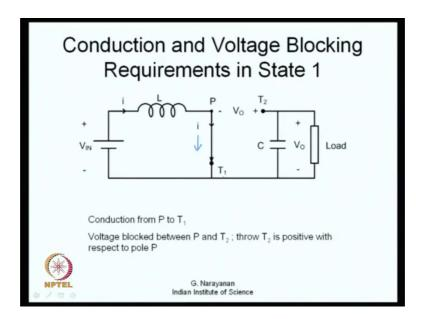
Let us look at the individual states one by one, if you look at the state 1 pole is connected to throw T 1 what is the direction of current? The direction of current is like this the current has to flow from P to T 1, and between P and T 2 whatever switch is connected that switch is in the off state. So, what do you have? You have a polarity where T 2 is positive with respect to P what comes between P and T 2 is the load voltage V naught.
