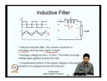
So, the solution is to go for an inductive filter; with an inductive filter what happens it smoothens down now.
