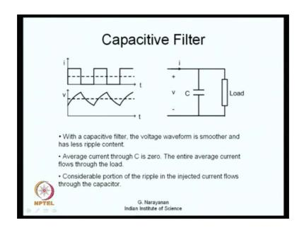
In an earlier in the earlier scenario when we applied voltage pulses here and wanted a smooth current we had an inductive filter here. Now what we have we are injecting current pulses here and we want the voltage to be smoother. Therefore, what we are trying to do is we are connecting a capacitor across that.
