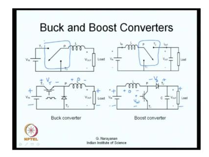
We need a particular kind of a single pole double throw switch that is one part of it and the enxt part of it is to understand how a particular single pole double throw switch can be realized.
