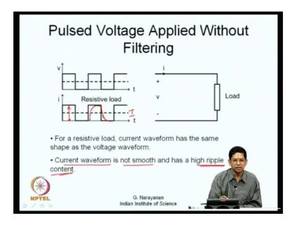
Now, let us say a pulsed voltage is being produced by a network of switches, there is DC source available and there is a network of switches. So, by switching this you are able to produce voltage waveform like this now.
