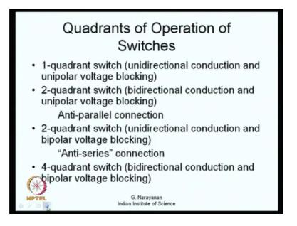
So, in this what we have is we have a transistor which can conduct in this direction, what we have done is we have taken a diode which can conduct in this direction, we have connected them in such a fashion that the transistor conducts in one direction, and the diode conducts in the opposite direction, hence we call this as anti-parallel connection.
