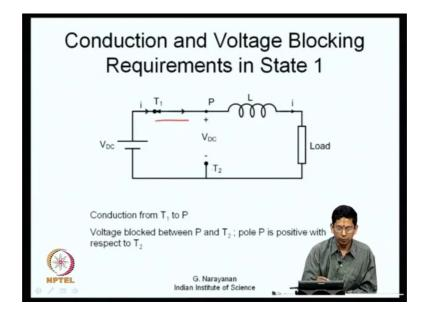
So, we move on we take a look at the state T 1 now. So, what do we need in state T 1 pole P is connected to T 1 it. So, you have certain requirement for conduction, whatever switch you may use between T and P 1, it should be capable of conducting in this direction from T 1 to P the direction of conduction required is from T 1 to P, when P is connected to T 1 there is no connection between P and T 2.
