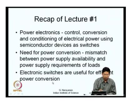
So, here is a quick recap. So, we dealt with power electronics. So, what is power electronics? It involves control conversion and conditioning of electrical power using semiconductor devices as switches.
