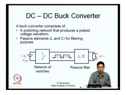
So, a DC what we desire from a DC to DC buck converter something like this, what we have is a DC power supply. And we finally, have a load here and this load needs a voltage this output voltage and this output voltage is much less than the input voltage is as less than the input voltage that s what we are we want now.
