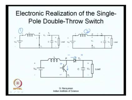
From this let us say we move on to an electronic realization of the single pole double throw switch what I have done is this is the state one this is state two both have been indicated here what you need between P and T 1 you need something that can conduct in this direction. So, you can use a transistor which conducts from its collector to emitter and which has to block a potential plus minus as indicated here.
