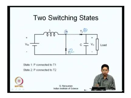
Let us look at the two states the converter in the converter there is only one single pole double throw switch, the pole P is connected to throw T 1 that is state 1 or the pole can be connected to throw T 2 that we can call as state 2. So, these are the two states now.
