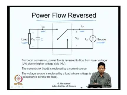
We want the power flow to be reverse how do you reverse this power flow? What we had here when it was load is basically a current sink now, let us change this current sink to a current source.
