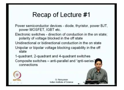
So, let us see more about switches, there are various power semiconductor devices available such as the diode the thyristor or the ac r on, the power BJT power transistor, bipolar junction transistor otherwise called power transistor and we have the power MOSFET, and we have the IGBT and you know IGBT as we saw in the last class it resembles a MOSFET in the when viewed from the gate side or from the viewed from the control side, when viewed from the power side it resembles a transistor now.
