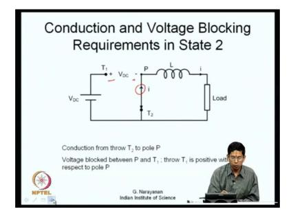
If you look at the state 2 it is slightly different, pole is connected to throw T 2. Now the direction of conduction is as indicated here, it conducts from T 2 to P the other switch which comes between P and T 1 is actually half now, and this blocks a voltage and this voltage is you know T 1 is positive with respect to P, the entire V DC comes across T 1 and P.
