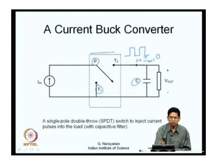
So, let us move on to how a current buck converter should look like, what we need is we have a load and with capacitive filtering we have a load and there is a capacitive filtering here and we can have such kind of a single pole double throw switch. The current source one of its terminals can be connected to the throw P, its other terminal I mean the pole P
