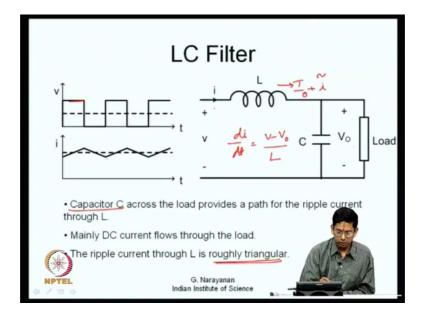
A further improvement is possible if you go in for an LC filter, now you still have the same pulsed voltage waveform applied, you have an inductance here in addition to that you also have a capacitance now.
