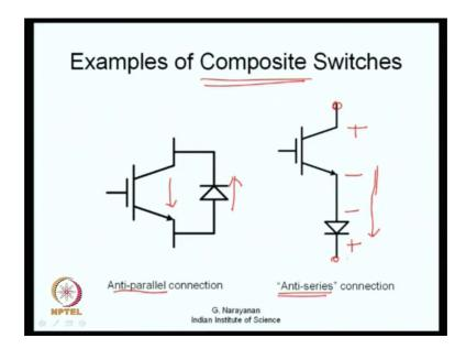
So, now here are some examples of first is an example of what is called as an antiparallel connection.
