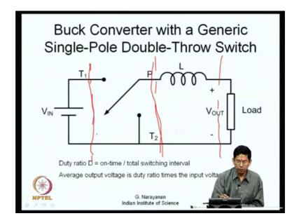
So, this is the switching network we are looking at and this part is the filter of course, in the filter I have ignored the capacitance c which you know may or may not be there. In application such as power supplies it is typical that the capacitance is there, where as in certain applications such as DC drive you might not need a capacitance here now.
