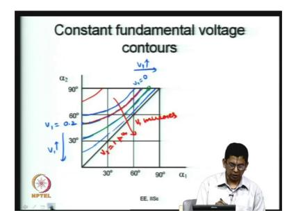
So, we were looking at how the fundamental voltage is vary, this is how the vary that is along this line on the alpha towards is alpha plane any point on this line gives you 0 fundamental voltage and any point on this line gives a 0.2 per unit fundamental voltage where one per unit stands for the fundamental voltage equal to the square wave operation there are the 6 step operation of the inverter now.
