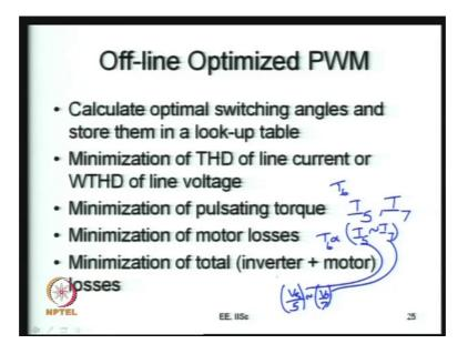
So, you can do an offline optimization you can calculate the optimal switching angles.
