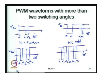
So, if you are looking at this is only up to 2 switching angles now you want to go more than 2 switching angles because this 2 switching angle you must realize that we took it up only as a means to improve or understanding. We just wanted to understand the relationship between the fundamental voltage and the harmonic voltages on one hand with the switching angles on the other hand. So, we kept the problem simple by only 2 switching angles now.
