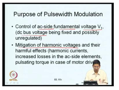
So, this purpose of pulse width modulation is what we want to do is we will have the DC voltage being fixed are you know may be unregulated regulated or unregulated whatever. So, it does not vary by itself. So, I mean it cannot be controlled we want to control the AC set fundamental voltage the question is how to do that. So, the pulse width modulation should help us achieve that desired amount of fundamental voltage now that is something that pulse width modulation is should help us now.
