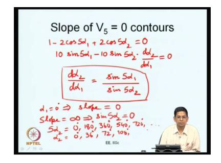
So, V phi is equal to 0 has this equation 1 minus 2 cos 5 alpha 1 plus 2 cos 5 alpha 2 is equal to 0 this is the equation V phi is equal to 0. If you want to find out the slope differentiate both sides with respect to alpha 1. So, what we are going to get is something like 10 times sin of 5 alpha 1 minus 10 times of sin 5 alpha 2 multiplied by d alpha 2 upon d alpha 1 is equal to 0.
