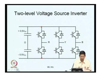
Instead of looking at it as generic switches if you look at it at actual width actual transistors and diodes this is how the circuit looks like. So, every leg has basically 2 transistors with antiparallel diodes and these conducting both the directions and they block voltage in just 1 of the directions as we have seen number of times before.
