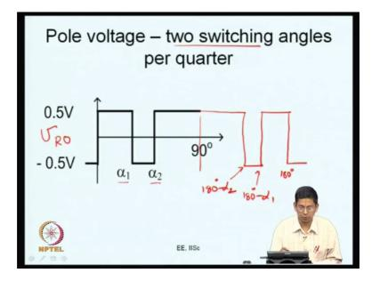
So, what we have been doing us first if you look at a square wave or you can look at just 1 switching angle per quarter cycle you can control with square where you cannot control the fundamental voltage, with 1 switching angle per quarter you can just control the fundamental voltage and you cannot influence the harmonics.
