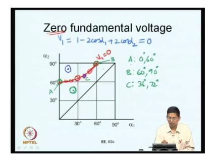
So, this is the bounds within a switching plane. Now for example, if your desired fundamental voltage is 0, the fundamental voltage has this relationship V 1 is equal to minus 2 cos alpha 1 plus 2 cos alpha 2 equals 0, I mean this is for the 0 fundamental voltage.
