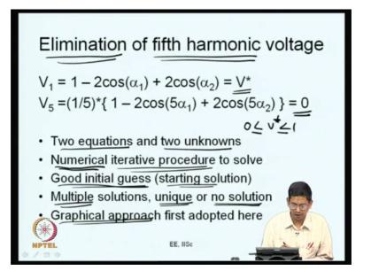
So, what goes without saying is if you want to reduce can it straight away make it 0. So, fifth harmonic voltage is the most problematic voltage in the sense that for a given amplitude fifth harmonic voltage will produce greater amount of the highest of greatest amount of harmonic current among all the harmonics is just 5 7 11 13 and etcetera. So, I want to reduce.
