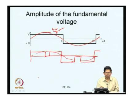
So, what is the amplitude of the fundamental I once again as I told you this amplitude of the fundamental is for such a waveform it is going to be the peak value is going to be four V by pi. So, this is the amplitude now, you cannot vary this amplitude if you want to vary this amplitude we should vary V; that means, the dc bus voltage is being varied, it is not the case that we are considering. We want you know V to be fixed. So, what we have
