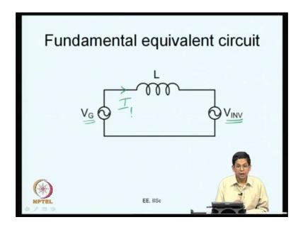
So, if you are interested in the fundamental current you want to see how much fundamental current is drawn the ripple voltage produced by the inverter makes no sense here they are at various frequencies. So, what you have is the grid voltage and this side what you have is the inverter output fundamental voltage, the fundamental voltage in the inverter line side and then the leakage inductance comes in between. This circuit helps you calculate the fundamental component.
