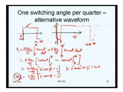
So, what we do in the earlier case was a situation like this. Let me just change the color to red here. So, the waveform was switching at zero degree and it is switching back at an angle alpha and this is 90 degrees. On the other hand, one could also consider a different kind of a waveform namely something that switches from high to low and low to high and still about 90 degrees. First let me indicate the horizontal and the time axis now. So, this is the voltage axis, this is the time axis now.
