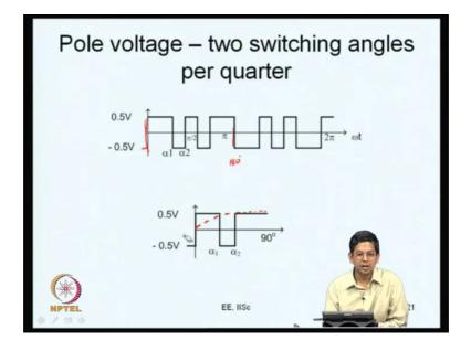
And let us move on from here to the problem of let us say two switching angles per quarter. The difficulty with one switching angle per quarter is you cannot control the harmonics, you can control your fundamental voltage, but you cannot control your any harmonic. So that is why you require a minimum of two switching angles now. So, here again what I said is this is the complete pole voltage waveform, I have just plotted it ready electronically, so that you know it is ready for us to see.
