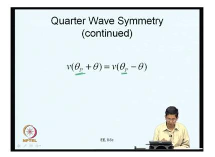
So, it is not exactly at 90 degrees. So, you can consider any theta p theta p is an instant where the fundamental component of the waveform V has a positive peak or a negative peak. So, it could be theta is equal to 90 degrees or 270 degrees going by our convention now. So, about this so you can say that V of theta p plus theta is equal to V of theta p minus theta this is what we have for quarter wave symmetry.
