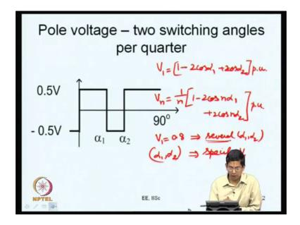
So, we have the same waveform reproduced here for just one quarter. And what is the fundamental voltage, we can say that V 1 is going to be 1 minus 2 cos alpha 1 plus 2 cos alpha 2 in per unit terms, this is what it is. And the n th harmonic component V n is going to be 1 upon n times 1 minus 2 cos n alpha 1 plus 2 cos n alpha 2 in per unit terms, again
