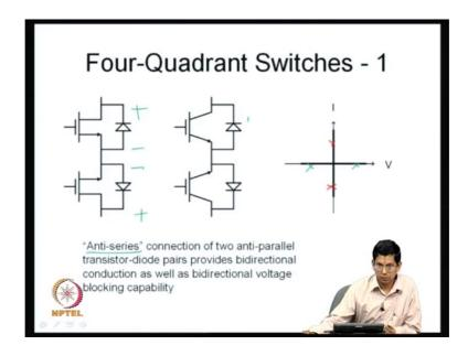
One simple way is; you already have an anti-parallel combination of a transistor and a diode to give you a bidirectional current carrying capability. So now, it has a unidirectional voltage blocking capability. Now you have to take another one, flip it around and connect it in series. And once again what I call as an anti-series, connection just you know it is a question of terminology to have an effective communication. Let us call the anti-series.
