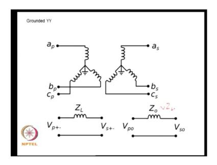
So, what is shown over here is see a Y Y transformer, where both the Y points are grounded. So, if you look at the positive and this negative sequence model going from your primary to the secondary, if you now do a per unitize analysis essentially the transformer becomes transparent. So, essentially you are modeling the leakage inductance and the winding resistance, the leakage inductance term is a dominant term.
