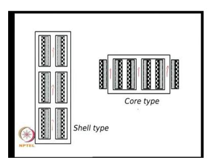
So, for example, if you look at a transformer you are familiar with core type or a shell type transformer. So, if you have a shell type transformer and if you have a 0 sequence flow that can flow in one of the windings, the windings of the primary or secondary winding of the transformer, essentially you will end up with 0 sequence flux. And the
