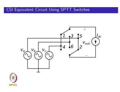
So, you could see that in this particular configuration your top single pole triple throw switch would be either in position 1, 3 or 5, which means that 1 and 3 is never shorted together because the pole would be only at one of this three points. So, which means that your voltage source would never get short circuited. Similarly, your top throw would be
