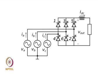
Again 4, 6, 2, 1, 2, 3, are essentially the switches, which is, which could be the thyristor or GTOs which would be fired, and typical firing sequence would be 1, 2, 3, 4, 5 and 6. So hence the labeling 1, 3, 5, 4, 6, 2 for the, for the switching devices.
