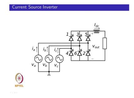
So, the previous power converter can be modeled as a pole connected to 3 throws on the top, and similarly a pole connected to 3 throws on the bottom.
