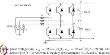
Nove the inverter legs assuming light load operation and sine triangle modulation.
