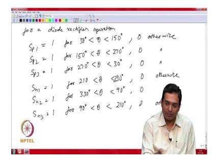
So for when it is operating without any delays, firing delays, etcetera for the thyristor, your S p would be on, S p 1 would be on for 30 degrees less than theta, less than 150
