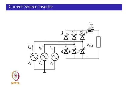
So, if you look at typical current source inverter, you have thyristors or GTOs connected. So, you need reverse blocking devices 3 phase, so you have voltage V a, V b, V c, current i a, i b, i c. Your DC link has a large inductor which emulates a current source, and the output can be a load or it can be a source when you need regeneration or breaking and you could then, write down the expression for the voltages.
