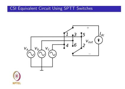
So, you have essentially a switch which could link 0.1 to the top or 0.3 to the top or 0.5 to the top or you could link say 4 to the bottom or 6 to the bottom or 2 to the bottom.
