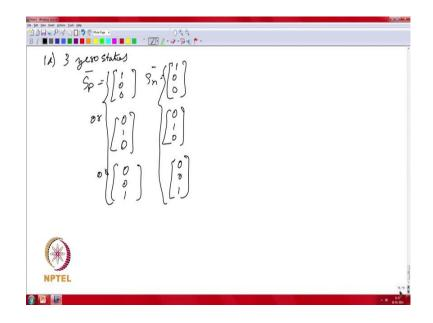
So, there are three possible 0 states, and unlike in a voltage source inverter where there are two 0 states in a current source inverter. There are three 0s possible 0 states, to look at the input output relationship between your AC and AC voltage. And the output DC voltage and also the DC current and the input AC current, you could write down the relationship.
