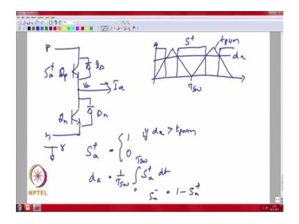
So, we considered switch in parallel with the diode this is transistor Q p and Q n and switching is S plus for say, if you have consider this as a and this is i a current flowing
