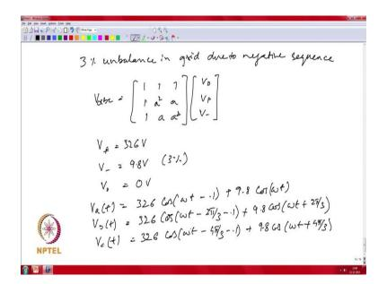
So, we have v a b c is and we have already to be 326 volts, it is continuing to operate under the nominal positive sequence voltage, your negative sequence voltage is 3 percent. If that corresponds to 9.8 volts and your zero sequence, you are assuming that to
