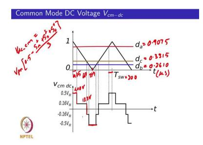
So, you have V dc common mode is equal to V p n into 0.5 plus minus, so if you plot that and all the switches s a, s b and s c are pi, then you have 0.5 minus a h minus 1. So, that would correspond to the duration over here, you will end up with minus 0.5 V d c
