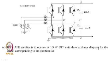
So, in the next problem you are asked to look at what would be the actual voltage at the a b and c terminals with respect to ground. The active front end rectifier is operating at 10 kilo watt unity power factor, by drawing a phasor diagram of this particular circuit.
