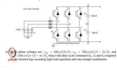
So, we will first look at the problem of three phase three wire power converter and it is operating as a active front end rectifier and it is connected to low voltage a c grid 400 volts with filter, inductive filter for interconnection. The filter is 0.1 per unit or 10 percent inductance and the switching frequency of the power converter is 5 kilo hertz and the DC bus voltage has nominal value of 800 volts.
