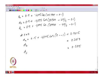
So, your duty cycle for leg A is now given by 0.5 plus 0.4095 cos 2 pi 50 t minus 0.1 and your d b is at this you can evaluate at time t equal to 0 and you get at t equal to 0. So, this would correspond to the value of duty cycle at time t equal to 0 and assuming that you have a digital controller, this would be the value that is used by the controller to compute
