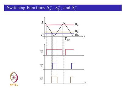
You can actually plot that, you have if you plot the carrier and the modulating wave forms d a, d b and d c.
