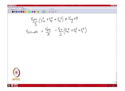
So, you could make use of this expression and substitute that in the expression one for the common mode dc bus voltage to get V dc common mode. So, you can express it in terms of your dc bus voltage and the switching functions of the individual legs, so if you plot it, you will get a function that looks roughly such a like this.
