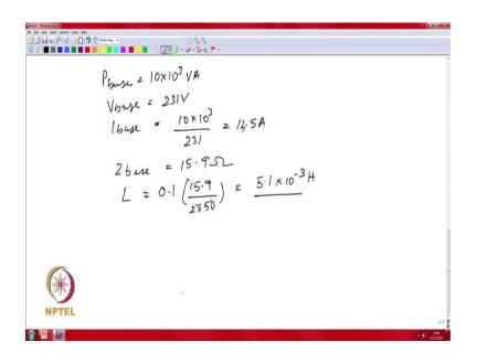
So, you have P base is 10 cube V A, 231 volts and I base is 14.5 amps, your z base is V base by I base. So, that is 15.9 ohms and your L filter inductance is 0.1 times 15.9 divided by 2 pi 50 is a fundamental frequency, so this corresponds to 5.1milli Henry.
