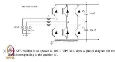
So, you have this particular voltage at when you are operating a 10 kVA, you can use that to find out what is a actual duty cycle that is commanded with a legs of a power converter.
