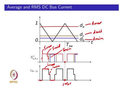
If you look at the speed of repetition, you would have essentially the switching period would be the period corresponding to when you have similar way for they are not exactly similar, because the duty cycles are changing over the sinusoid. You could think about the high frequency component repeating at 5 kilo hertz or t s w.
