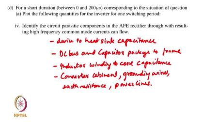
So, device to heat sink capacitance, then the split and capacitor package to frame capacitance, you have inductor winding to core capacitance and you have your actual converter frame cabinet, your grounding wires, your earth back through the power lines. So, this would form a loop through which you could have common mode currents flowing which would lead to interference phenomena.
