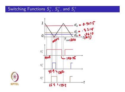
Your d a intersection would correspond to 9.25 going on till 190, your b t, b switching signal would correspond start from 73.9 up to 126.2 and your switching function of AC would be between 66.8 to 133.2. So, you could actually find a instance depending on the duty cycle and your triangle your carrier. So, this would be 200 micro seconds, this
