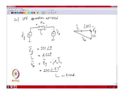
So, for UPF operation, unity power factor operation at 10 kilo watts, you have your grid voltage e g phasor, then you have your filter inductance with the current to the filter being ideal and you have phase a voltage phasor V A which you want to figure out. So, if we have the phasor diagram would be you are your grid voltage and you have the
