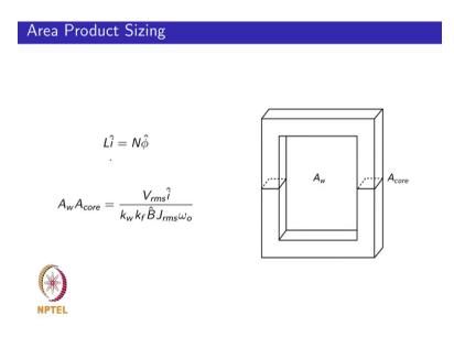
So, when you are considering the area product of the filter you are essentially looking in this particular case you have to looking at double c course. So, there is a upper c and a lower c structure and essentially you are looking at the product of A, the window area and the core area cross sectional area of the core. So, to derive the expression for the area product you start off with the definition of inductance which is the flux linkage is proportional is given by L i in the inductor.
