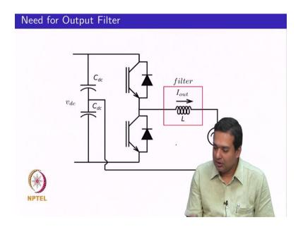
So, if you have say transients in the grid you have also constraints on how much fundamental voltage drop would occur across a filter inductor and which can then influence the amount of d c bus voltage that is required you also have. So, if you have a large value of L the dynamic response to the system would be relatively sluggish, so we know that if the inductor is too large.
