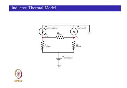
So, one could then also look at a slightly more sophisticated model of the of you of your thermal model of the inductor one can consider thermal resistance between your winding to ambient. So, you could consider thermal resistance from your core to ambient, you could also consider because the winding and core is mounted close by. But, you could have conduction paths or small air gaps through which you might have heat transfer between a winding to your core.
