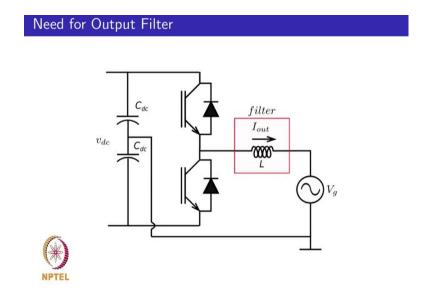
There is a primary requirement of minimizing the amount of ripple that can be sent out into the grid and there are standards such as I E E E 5 1992 and I E E E 1547 which provide recommendations on the level of harmonics that can be injected into the grid. We can also then last time we saw how we can derive an expression for the peak to peak ripple current.
