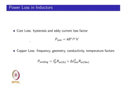
So, the power loss in the inductor is actually a important factor the power loss in the inductor correspond to two factors, one is the core loss that is happening in the magnetic material and the copper loss that is happening in the windings. So, and one looks at the core loss the dominant terms are the hysteresis and eddy current loss factors and when you look at the core loss in a material it depends also on the type of material that one would select for the core.
