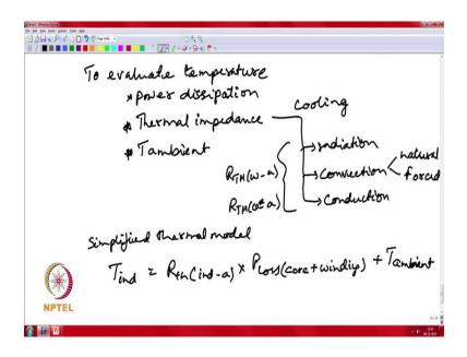
So, one is what is the power dissipation the second aspect is the thermal impedance and the third factor is what is your ambient temperature. So, your actual operating temperature of the your inductor would depend on all these factors and we are just discussing about the power dissipation.
