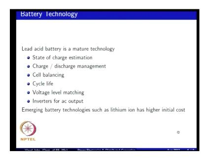
If you look at specifically the battery technology there are many challenges in batteries the lead acid is a mature technology today and cost wise it is quite competitive compared to the other challenging battery technologies. However they are challenges of how to estimate the state of charge for example, if you are using it in a vehicle application you would like to know when your fuel gauge is empty or whether its full.
