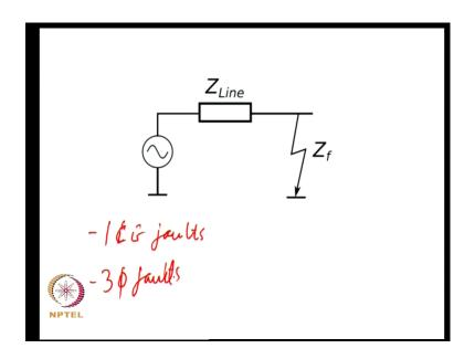
If you look at the model for a typical line this is what we just discussed and if you look at what happens during a fault such as a insulation fault or some sort of short circuit fault you can have different varieties of fault depending on a fault impedance. So, the question is you what numbered you use for typical values of say the fault impedance inner fault scenario.
