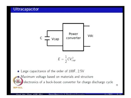
If you look at the ultra capacitor as a energy storage element people are looking at ultra capacitor closely today, because its ability to charge and discharge much higher than a battery. So, people are looking at possible combinations of ultra capacitors and batteries to be able to rapidly charge and discharge energy. So, compared to a regular capacitor these ultra capacitors would can have, much higher value of a capacitance.
