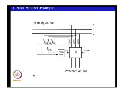
So, the question is now, with this, how to make use of it for operating protective device? And we look at an example, where you have a simple example of a three-phase circuit breaker. So, in here you have say a three-phase AC circuit breaker -52 – you have an
