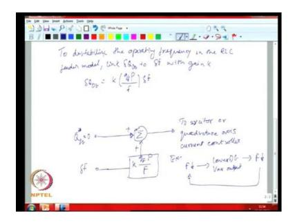
You could link your reactive power to change in frequency that is measured in the DG, so essentially what you would do is change your output of your DG with some gain times q quality factor power operating frequency with delta f. So, you could think of essentially your block diagram as on the nominal conditions q DG command would be 0.
