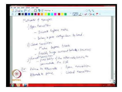
So, methods of transfer, one is called a open transition, in open transition essentially it means that to transfer from one source to other, first you open both the switches and await for small for the small delay to ensure that the switches are perfectly open. Then, you turn on the switch for which you want to transfer to, so here you are having a break before make operation and here the delays can be longer. The power poorer voltage would be seen by the load for a longer duration.
