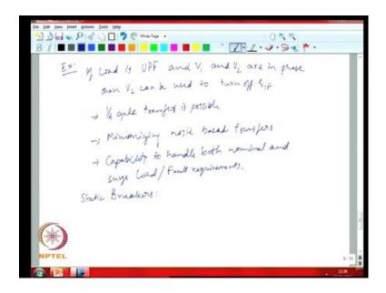
So, say if the load is load is unity power factor, so if you assume it a resistive load V 1 and V 2 in phase and then you could think about operating in the positive half cycle of the voltage. If it is under that particular condition, if the prime source voltage went away because of an outage.
