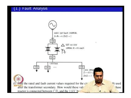
So, the next question is what would be the rated current and the fault current level of this 8 circuit breakers that are protecting the feeder, and the second part of the question is what would happen if you add a impedance in series with circuit breaker 1 on the 11 on the low voltage bus.
