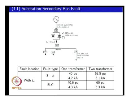
And, you can see that now which the reactor your fault current level with the 2 transformer case it reduces to about 6.3 kilo amps, with 1 transformer it further reduces. But now, compared to the previous case where you had 11.8 kilo amps as the fault current level of circuit breakers to through 9, now you have circuit breakers which need to interrupt 6.3 kilo amps.
