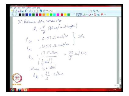
So, the resistance is by row by A, where this is in ohms per unit length. And row for copper is ohms per annum square per meter, and row aluminum; this is at 20 degree centigrade, your resistivity is v of function of temperature. And so you can write your
