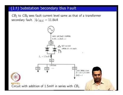
So, then the next part of the problem is what would happen if you now add a reactor of 1.5 milli Henry in series with the low voltage of the, in series with circuit breakers CB 1. So, you can see that essentially adding a reactance over here will now reduce your fault when if you have a fault immediately downstream. So, you could now do the calculations of what would be the fault current level, now which the circuit with this particular reactor.
