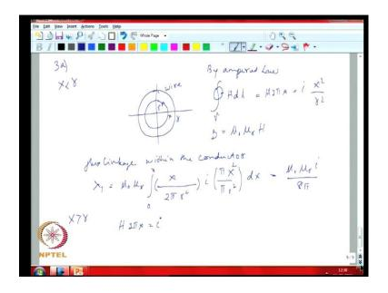
So, to determine the reactance of the line you are looking at the inductance, the flux linkage of the line. So, if you have a round conductor of radius r; and you have look at 2 cases- one is what about the flux linkage within the conductor and the flux linkage outside the conductor. So, when you look at the first case where you are looking radius x less than r. So, you are looking at the flux linkage within the conductor, and say you have a close path gamma and this is the wire on conductor.
