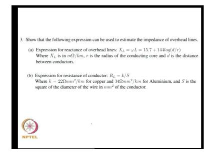
So, in the next problem we are looking at over headlines, and looking at its resistance and its reactance, and you are asked to look at obtain expressions for its reactance and resistance based on its geometric parameters. So, the expression for the reactance of over headline is something that is available from book on, textbook on power system analysis. We will just briefly go through that and write down the expression.
