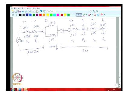
So, you have the source which is 1 per unit. So, you have your transformer primary bus, you have say breaker, you have the leakages of the transformers. So, you have the low voltage bus at the substation; then you have your breakers that protect each feeder; then you have the reactance and the resistance of each section of the line.
