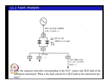
So, the next problem is find to, normalize the system, permutize the system using the 2 MVA base of the feeder.
