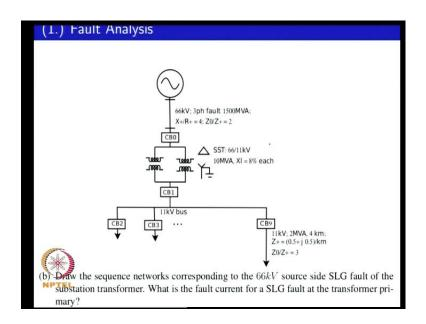
So, in the next problem you are asked to draw the sequence network and find the, what would happen if you had a single line to ground fault on the substation transformer on
