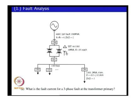
So, we will look at first problem where you have a 66 kv sub-transmission line feeding say a substation consisting of 2 transformers; you are given the fault MVA at the transformer primary 1500 MVA. You are given the X by R ratio for positive sequence, and the ratio of the 0 sequence to positive sequence impedance this is 2. You are given the rating of the transformer; it is 10 MVA, 66 KV slash 11 kv line to line. And your leakage inductance is 8 percent each.
