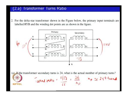
So, next problem is about delta y transformer, and the primary voltage is 66 k v, and your secondary voltage is 11 k v on a line to line basis. So, if you look at your secondary which is Wye your voltage on your winding is 11 divided by root 3. So, you could calculate; so the first question is to calculate what would be your primary turns if your secondary turns is 24. So, you have the turns ratio; your n p is about 249 turns.
