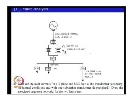
So, the question is what are the fault current levels for a 3-phase and single line to ground fault at the transformer secondary, for normal conditions being when both transformers are available at the substation; and the second case is when one of the, one transformer is de-energized may be for some repairs or maintenance, draw the associated sequence network for these 2 fault cases.
