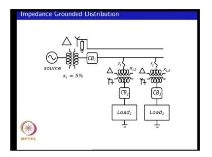
So, we are talking about having a impedance now connected between the neutral of the transformer under y side and the earth, the earth in terminal and it can be a resistance or a reactance. You can have the possibility of high impedance or low impedance grounding and we saw in the last class an example of a small value of reactance, which is connected between neutral and the ground.
