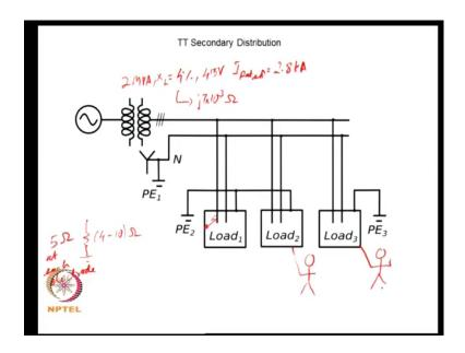
You could actually calculate what your touch potential is say if a person is over here and the person say if he touches load 2 because you now have a current flowing through power earth 2. You have a resistance between your earth and there is a contact resistance the frame of load 1 and load 2 will get elevated when you have a single line to ground fault and you could calculate what that particular voltage is.
