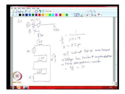
So, we will look at example of high resistance grounding, so we will look at an example where you have a source and say this is delta y and the y is connected through a resistance of a say 5 per unit. You have a circuit breaker and say the impedance X L of the transformer is say 5 percent and you have a single line to ground fault occurring somewhere down the distribution line.
