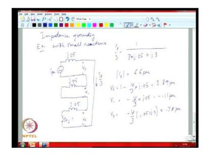
So, we look at impendence grounding and you look an example of j point 1 per unit as we mentioned. So, if we look at what would be the resultant sequence network, when there is a fault, so the positive sequence network is this is a negative sequence network and then assume ZF to be 0 and the current here is IF by 3. So, you can see that your fault current level has come down, when we had side grounding plus 20 per unit, now IF is 6.6 per unit and then we can look at a resulting voltage V plus.
