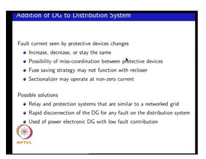
So, if you have fault current level changes, during to the addition of a distributed generated source, then there is a possibility of miss-coordination between your upstream and downstream device, because of this change into the current level. And you cannot uniformly say that the current level is always going to increase, at the protection point it can actually go in all three ways.
