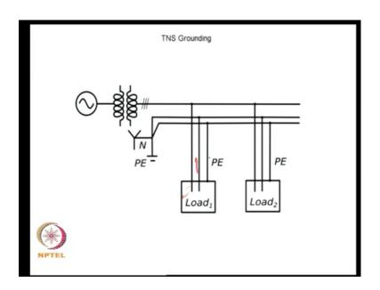
Where, the neutral and the power earth are now separated as conductors, so your unbalanced load currents will flow through neutral conductor and only your fault current will flow through your ground conductor. So this is a TN with separate ground and neutral conductors, here it is now possible to differentiate between a case of unbalanced and ground current, but here again you can see that immediately the cost is high for distributing a power in three phase, when you have five conductors.
