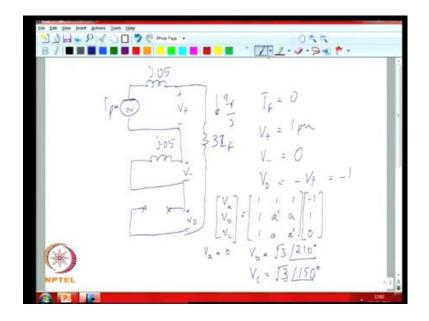
So, you have your positive sequence network, so in this particular case we had assumed that you have a transformer with 5 percent reactance and the zero sequence network is actually now open circuit, because it does not grounded. So, if you look at the there can be no fault current in this IF should be 0 in this particular case. So, you have V plus is equal to 1 per unit and V minus is 0 and V 0 is 1 minus V plus minus 1, so then if you look at your phase voltages using the sequence transform.
