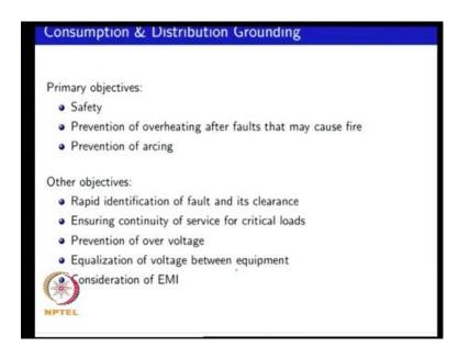
Now, we will look at any another aspect of the distribution system important factor again, it has implications when a DG gets connected and that is grounding. So, if you have a any electrical system you would ground it and the primary objective of grounding of a system is actually a human safety, someone should not touch electrical system and get a shock you should not get electrocuted.
