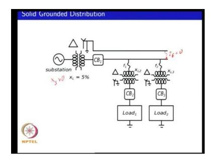
So, the next possibility is say instead of having a insulated or an ungrounded source you could actually have a solidly grounded source. So, this is an example where you have a delta Y transformer which is acting which Y is now your source and the neutral is now connected to ground through no intentional impedance and for the analysis, we assume
