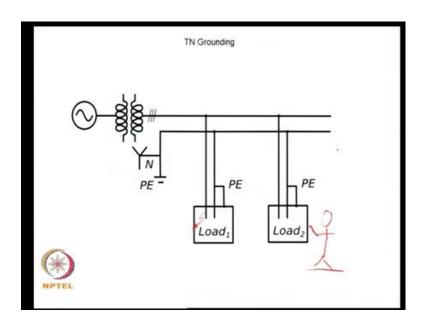
So, if you look at them an example, system were you have a solid line solid line to ground and in solid grounding of the source, an example is that TN network, where the Y point of your transformer is solidly connected to power earth and the neutral is then distributed to all the loads and so that the neutral is now expected to be up low voltage at the ground voltage, because it is connected in a tight manner to power earth.
