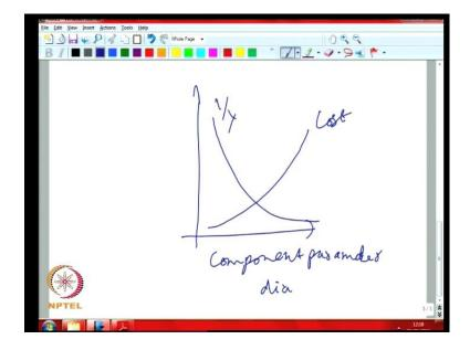
You are looking at a say a tradeoff such as a some component parameter, such as the diameter and on the one hand if you are looking at the if you are increasing the diameter your cost is going up. But, your mean time between failures say 1 by lambda would actually come down because you are having a more reliable component, so you also have this tradeoff between reliability and cost. So, if you are designing a power electronic component and you wanted to lost for, so many years.
