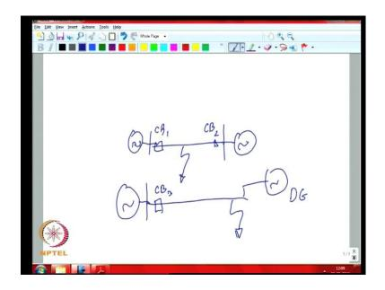
Then you have a scenario, where say you have two sources, suppose you have a fault over here at the center of the line, then to clave the fault you need to actually open say breaker 1 and breaker 2 to actually clear that fault. Because, just opening one breaker is not sufficient, you need to disconnect all the sources to actually clear the fault, if you look at the traditional distribution system, you might have a breaker at C B 3 and say you have a fault somewhere down on the feeder.
