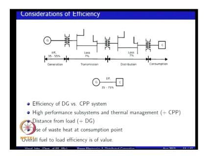
If you look at the issue of efficiency of a the distributed generation versus the centralized generation, you can have a variety range of efficiency over here depending on the type of plan, whether it is a just a boiler or running a turbine or it is a got different stages of which can help improve efficiency or whether it is a natural gas power plant. Where you can have improved efficiency, you also have losses in transmission systems, losses in the distribution system.
