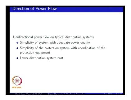
That the concept of unidirectional versus bidirectional power flow has a got a lot of implications, ((Refer Time: 18:50)) just again on the previous slide I just want to point out just because you have a lot of people associate distributed generation with solar energy or wind energy. But, that is not necessarily true all the time, I mean if you look at large wind farms they might be even though the individual turbine might be rated at
