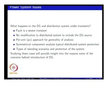
So, we talked about pre-aspects of a this course, so the first aspect was power systems related. And as we mentioned the fault is a severe transient and you need to actually deal with a fault in a power distributed generation system and one of the basic requirement would be that you have the existing distribution system with it is protection philosophy. And you do not want to modify the existing protection system, when you add in the distributed generation source.
