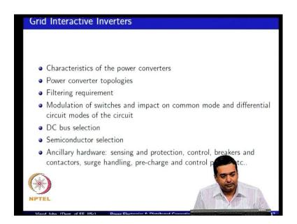
The third part of the course is about the power electronic details will be looking at the characteristics of power converters, the topologies, the requirement of filtering, the output of the power converter you do not want your neighbors, a computer to shut down every time, your solar panel under roof generates power. So, you want a tight filtering and you want it to be compatible with the things that are there around you.
