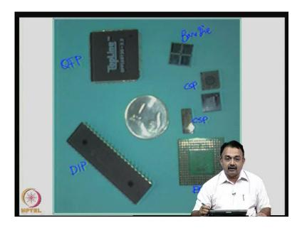
These components I have in my previous class tried to show you, but I have tried to put together here one single picture where you can compare it with our one rupee coin. This is our DIP package. This is the DIP package; then you have the QFP; then this is the BGA – ball grid array; this is CSP; these are the two sides – the bottom side and the top side of a CSP; this is a bare die.
