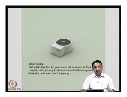
Finally, these packages will go for routine electrical test once again, especially in terms of power dissipation and frequency handling. These are electrical tests that will have to be conducted once the die has been packaged; only then it is qualified.
