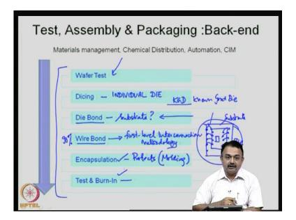
If you look at this flow chart, we are now at the back-end processing of the die manufacturing; this is known as test, assembly and packaging section. The first one was basically from the silicon to wafer. The wafer here is tested, as I mentioned earlier; test becomes very important in every step. I have written about six steps here, but in practice it goes through a very large line of subprocesses including electrical test, materials management, material analysis and so on.
