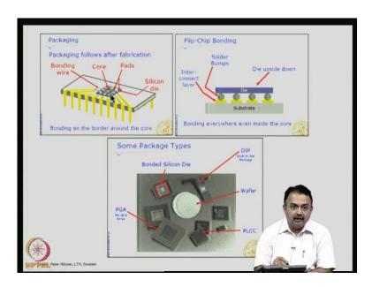
If we look at the slide here, briefly, you can see on the left we have here a substrate (Refer Slide Time: 11:56) – the lead frame – which houses the die that we have manufactured. Here, you can see on the die in the periphery various die bond packs that are marked in black. What you see here are the lead frames which connect to the outside world.
