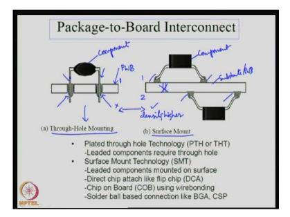
If you look at Package-to-Board Interconnect, basically this is second-level interconnect. If you look at this figure, this is your printed wiring board and this is your component – the package (Refer Slide Time: 46:09). These are known as through-hole packages. This component has leads which are very long and these need to be inserted through the holes present in the printed wiring board; so, these interconnection choices are known as through-hole mounting interconnects.
