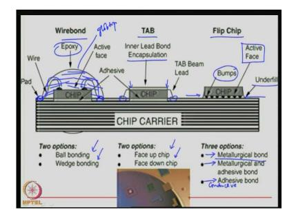
As I said in the previous figure, this is known as a glob top. This process here, what we have seen, is known as a glob top process. We use a glob top to bare die with epoxy resin (Refer Slide Time: 59:19).
