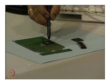
Now, we are going to use a printed wiring board like this and try to see how we can establish a connection from the first-level package to the second level. Connections on this board are known as second-level interconnections (Refer Slide Time: 45:45); connections here are known as first-level interconnections; I hope it is clear.
