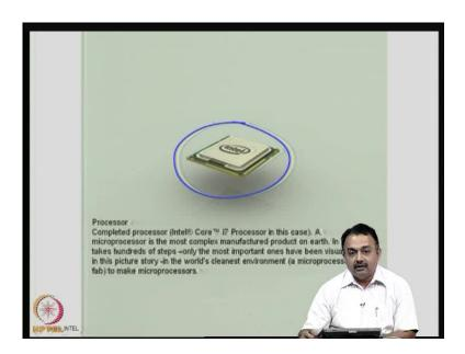
For the processor in this particular example flowchart that we have been seeing over the last two classes, the processor packaging is complete. The illustrations we have seen are very few, but in actual practice there are scores of subprocesses that the wafer has to go through including the back-end packaging, die bonding, wire bonding and so on to make sure that you get a more reliable package.
