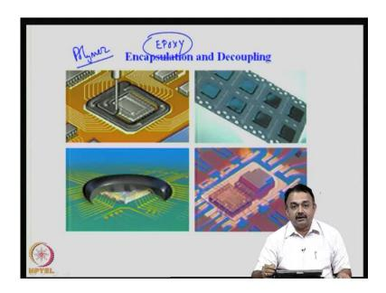
Now, briefly about encapsulation; encapsulation is basically a process of using a polymer material to protect the die from the external environment. What is the external environment we are concerned about? Temperature increase, dust and humidity. The polymer material should be inert; it should protect the wire bonds that you have established or the flip-chip bonding that you have established and protect the die from external influences.
