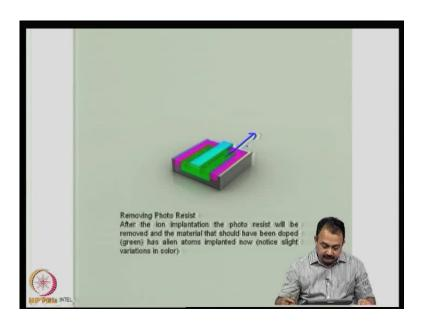
Now, once the job is over, you remove the photo resist and the material that should have been doped, green, in this case, has now got the dopants, the new material implanted; and you can see, there will be variations in the properties of these host material plus the dopant.
