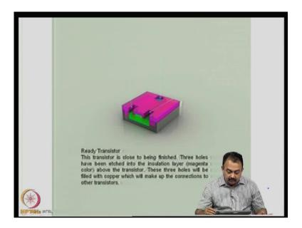
Now, the transistor is now close to being finished. Three holes have been etched on to the insulated layer; this magenta material is the insulating layer; you want to insulate it because that particular process is over; so you convert the surface into an oxide and then make a passive; so you make it convert it into oxide. These holes are generated now and these holes will be filled with the copper conducting material, which will finally, be the connectors for these transistors.
