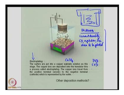
Now, how do you make this area conductive? The exposed area, as we seen in the previous slides, the open areas need to be plated with the conductor; typically, we are going to use copper. In this particular example we are taken up the process called electroplating.
