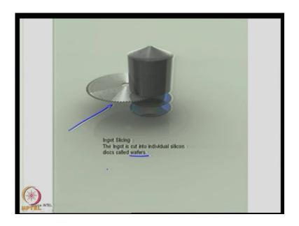
Now, the next step is we have to slice this ingots into individual silicon discs called wafers; that is a next process.
