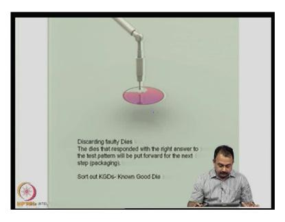
After the dies are singlulated, you get single dies now; and you have to qualify it has a known good die, KGD so, again you can probably do an electrical test for each of these dies and it can put it through a series of programmed testing, which will say whether this die has passed the requisite test.
