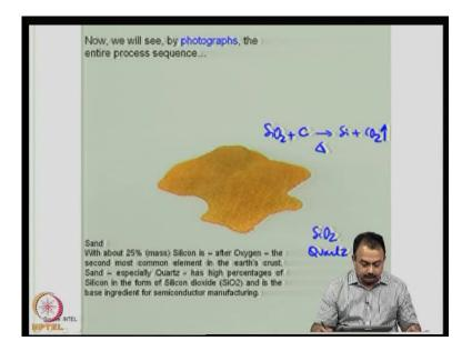
Now, how do you convert silicon dioxide to silicon?; that is the first step, right? Typically, silicon dioxide is made to react with carbon and this forms silicon plus carbon dioxide. This is the basic reaction and this happens as at higher temperatures. So, you get the first step of the formation of silicon.
