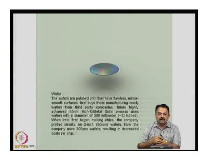
Now, the wafers are polished. Once you get the first cut wafers, before is start doing the imaging process on the wafer, you want to make sure that there is no defect caused by the cutting or extraneous material or surface defects. So, you want to polish it; and you can see that polishing can give you a very nice, mirror-like image, as you can see here.
