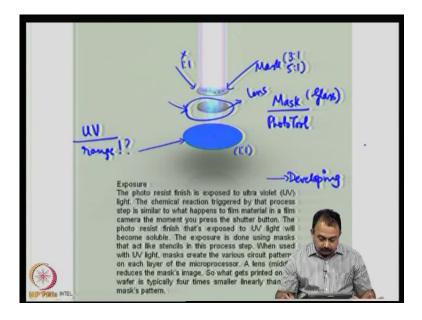
Now, we are talking about exposure; that is the next step. What is exposure? You are exposing this photo resist to UV light and when you exposing this, you are going to use what is known as the mask or the tool photo tool, typically made on a glass substrate.
