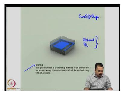
Then, once this photo resist, which is basically cured now, at specified temperatures so that it becomes very hard and it protects from certain areas on the wafer. Now you want to remove unwanted material in this stage, from the base substrate.
