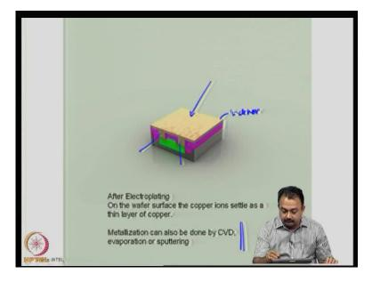
So, after electroplating, on the wafer surface the copper ions settle as a thin layer of copper, you can see here, very nicely, the entire surface has been covered with copper, including these areas, which define the transistors. Now, as I mentioned before,
