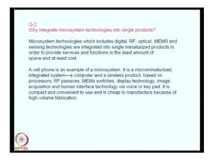
The next question that I am asking you is- why integrate microsystem technologies into single products? What is the need for having single products? Does it affect the size? Does it affect performance? So, microsystem technologies, which include digital RF, Optical MEMS and other sensing technologies. They are integrated into single products
