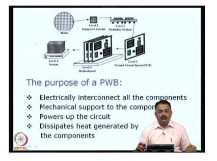
The purpose of a printed wiring board will be to electrically interconnect all the components, mechanical support to the components, powering up the circuit and it also dissipates heat generated by the components. So, naturally, you can expect the dielectric material used for the printed wiring board to be somewhat thermally conductive and remove heat to the atmosphere. You can also improve the thermal performance by adding heat sinks.
