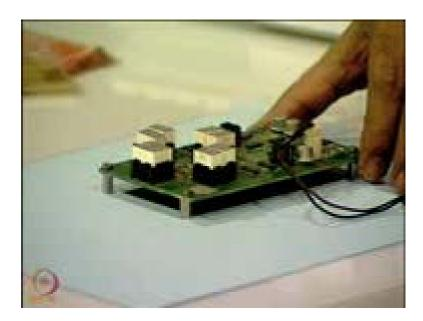
This is another printed circuit board, which is again mounted. You can see a lot of active devices, lot of displays on the board. So, this is also an organic substrate.
