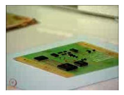
You can see in the figure or in the sample here, which I am showing right now is a printed circuit board. You can see various devices and all of them are surface mount. You can also see very tiny devices and these are all the resistors, capacitors and are in very small size. To handle these, you require equipment to pick, place and attach it on to the board. I will quickly show some other examples of PCB's.
