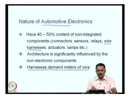
What is a nature of automotive electronics? As a design engineer, I think you must look into improving technologies in these areas. These are the current status and they have about 40 to 50 percent content of non-integrated components like connectors, sensors, relays, wire harnesses. This is going to take a lot of space under the hood and around the car actuators, lamps. Extra architecture is significantly influenced by the non-electronic components.
