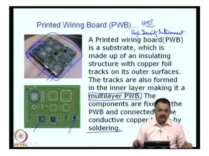
What is the printed wiring board? A printed wiring board is a substrate, which is made up of insulating structure that I showed you as an example with copper foil tracks on its outer surface. The tracks are also formed in the inner layers. I mentioned that you can make multilayers. So, the tracks need not be on the top. In the bottom, there will be inner layer, which connects to the top and bottom copper layers making it a multilayer printed wiring board with very high density.
