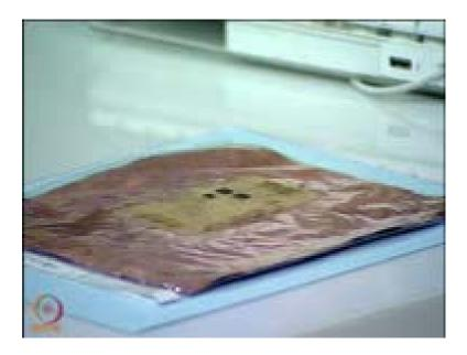
Now, I want to show you another example, a building block of a printed wired board. Now, this is a material that you are seeing here, which is the dielectric material that used in the building of the printed wiring board. This is made out of glass plus an organic resin. Now, on top of this, a copper foil like this will be laminated on to the base dielectric material to give a rigid board like this.
