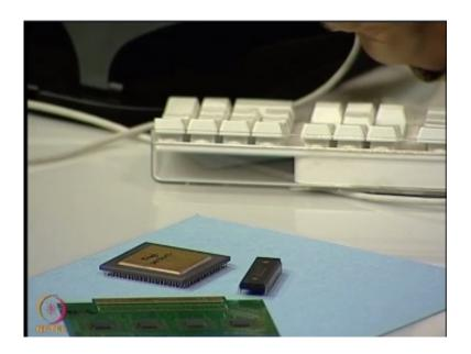
Then, you have Pin Grid Array or Column Package, which I have showed in the last class, the familiar Intel Pentium processor, which has the input output pins in the form of a pin, really thick pins as you can see. Now, you can see the pins. This is a single chip module. All these are single chip modules.
