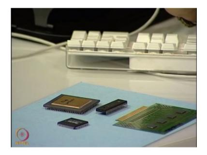
Then, we have the QFP, Quad Flat Pack or Package. What I am seeing here is a Quad Flat Pack because as you see, if I rotate this on all the four sides, you have the pins. The periphery of the package on all the four sides contains the pins. That is why it is called a quad, whereas this is a dual; so, Quad Flat Pack or Package. There are various types of Quad Flat Packages. We will see as we go along.
