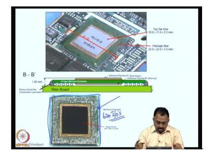
This is an example of the solder ball array. As you can see series of solder balls here, it is occupying the entire area under the die. This is the die and you can see how many? There are 620 I/Os on this particular example, which is very large. So, there are FPGA modules today, which come with 1200 I/Os, 1200 pins, which you have to handle efficiently without even a single error during assembly.
