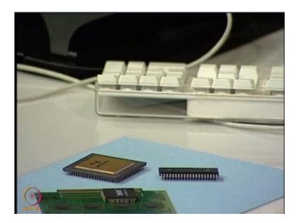
Let us now go to the other category – Surface Mount Package. In the Surface Mount Package, we have what is known as Small Out-line Package. As the name indicates, the Surface Mount Packages will not have or will not have a requirement of the pins going
