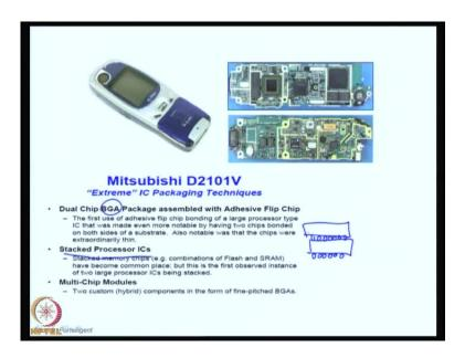
This is again new technologies used in current day cell phones, where people are using BGA packages to enhance the electrical performance; they are using stacked processors. That means one processor is stacked over the other by suitable technologies. So, 3-D packages are being used and Multi Chip Modules with low profile / low thickness is also being used. So, these are some of the examples that I can give, which shows change in manufacturing using new technologies at the packages level.
