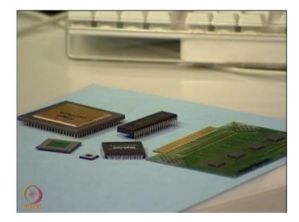
Finally, if you can have a look at it, these Multi Chip Modules will get some kind of a format of this type, but it can be smaller. This can easily go on to a motherboard. So, Multi Chip Modules can also be mounted on to motherboards. I hope it is very clear. Single Chip Modules after they are fabricated, they will be mounted on the motherboard. Multi Chip Modules also will get mounted on to the motherboard and then go through the process technologies as a Single Chip Module.
