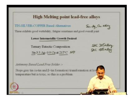
Now, we will move into high melting point Lead-free alloys; in this, specifically we will look at Tin-Silver-Copper based alternatives to tin-Lead soldering. Now, Tin-Silver-
