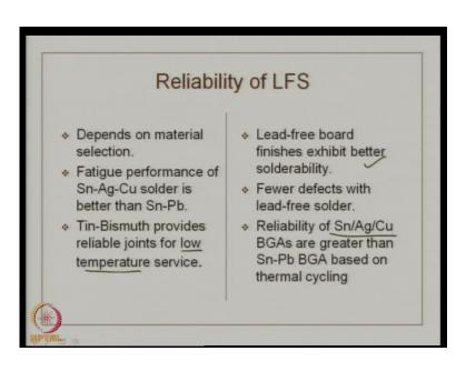
So, the reliability of Lead-free solders or soldering process as a summary depends on material selection. The fatigue performance of Tin-Silver-Copper solder is much better than Tin-Lead, as we have seen over the years. Tin-Bismuth provides reliable joints for low temperature service – low temperature assembly. Lead-free board finishes exhibit better solderability. There was a concern about the reliability issues, the wetting and the
