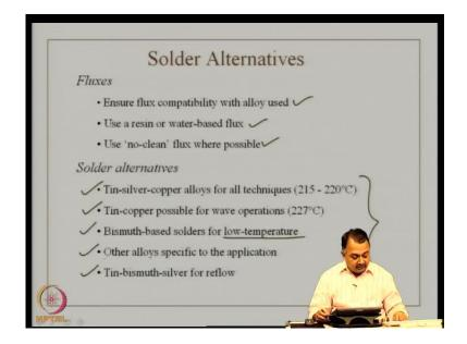
Now, from the solder side, it is very important that you are going to use fluxes or flux; it could be an inbuilt component in your solder paste. When you use solder paste with screen printing or stencil printing, you are going to use flux; you are also aware of noclean fluxes, but generally there are different fluxes like: mildly activated flux, low activated flux, and then super activated fluxes. You need to understand what kind of flux is being used in that particular process.
