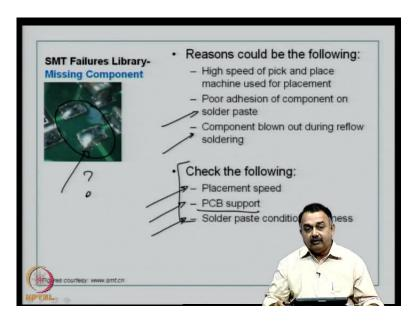
The other thing is, when you work with automated machines, the component could have been blown out during the reflow soldering. Again in a reflow, if there is convection air, the component is probably displaced because of the air inside the reflow machine. So, again it emphasize the fact that reflow soldering process when you use a solder paste, the solder paste should have good tackiness.
