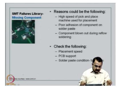
Next defect is, missing component. As you can see here, there is supposed to be a component here but that is missing. The reasons could be very simple. When you are doing an automated pick and place, this normally does not occur, when you do small volume prototyping manual placement but normally encountered with high speed pick and place machine that is used for placement of a large number of components and those large number of components could be very light chip components. When you place a
