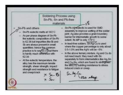
Now, we will look at soldering process using tin lead, tin and lead-free materials. We have seen with tin. Now, we will look at tin lead and others. Tin lead eutectic melts at 183 that is the composition of tin lead at 63-37, tin 63 percent lead 37 seven percent. The eutectic temperature is 183 C which is the lowest of tin lead alloys.
