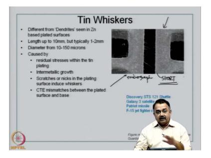
The physical parameters of these tin whiskers: typically they can grow up to 10 mm, typically about 1 to 2 mm very fast, diameters ranging from 10 to 150 micron. They are caused by residual stresses within the tin plating.
