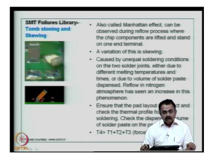
The next failure that we are going to see is Tomb stoning and skewing. What you see in this particular case is tomb stoning and this is skewing. This is also called Manhattan effect. It can be observed during the reflow process, where the chip components are lifted and stand on one end terminal.
