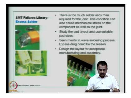
The third defect is excess solder, which means there is too much solder alloy, as you can see, than required for a particular joint. Because the size of the package is very small, you do not require too much solder. At the same time, you cannot have deficient solder too. This condition can be detrimental to the board because it causes mechanical stress on the component. Because there is too much solder, it can heat up the component, it can cross stress on the component material as well.
