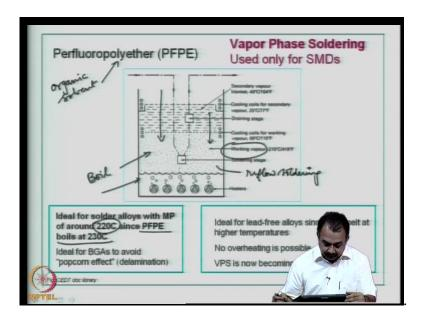
This is very ideal for BGAs to avoid the popcorn effect. In the Printed Circuit Board the assembly process can be done for a few boards depending on the area of the chamber. The reason why we say that this is ideal for BGAs is because you can work at temperatures that are not detrimental to the substrate and the solder ball attachment.
