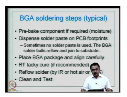
As a summary, we will look at writing down the soldering steps for a BGA. We have seen the various process mechanisms by which you can attach a BGA. I will just list the typical BGA soldering steps. First thing is prebake the component if required, remove the moisture the reason is you want to avoid pop corning effect.
