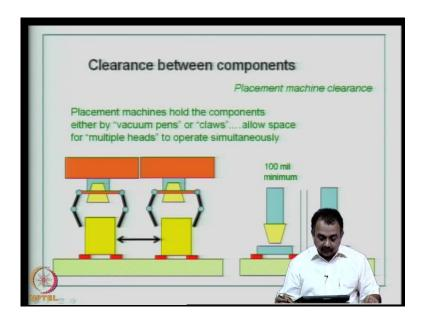
This is a design issue. If you look at clearance between components, again we are talking about a placement machine clearance. In some cases, the placement machines hold the components either by vacuum pens or claws as you call it and that requires a lot of space, as you can see here and it could be a very tall component. Therefore, you have to give a gap between tall components and it is not advisable to place any components here in the gap.
