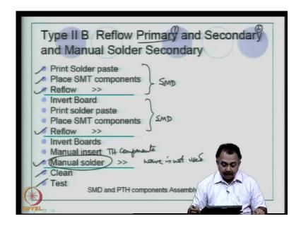
So this is known as Type II B. This basically says that kind of components in each of these, the first one you had a complete SMD, no through-hole components, the second one you had a few through-hole components that require wave soldering. In third type, you have reflow primarily and then a couple of through-hole components that can be managed with manual soldering. Even in this case, you can do manual soldering if you feel the percentage of through-hole components is much less.
