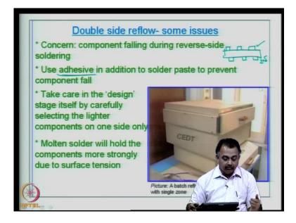
What I have mentioned are typically process steps for a single sided of assembly - very simple; there are no major issues; only thing that you have to make sure is that the temperatures are set; but when you do a SMD assembly on the Printed Circuit Board with SMD components on both sides, then you have some issues, which if you take care, will give you higher yields.
