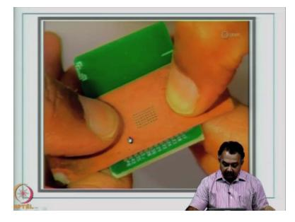
You have to align perfectly. After you align, make sure it is firmly held in its place by an adhesive or a tape. Now you are going to use a kind of a squeezing blade material. Here you can see this is the solder paste. The solder paste is now printed through the perforations representing the BGA solder balls and then the solder paste is transferred. You can see here the solder paste is transferred on to the copper pads of the BGA pattern.
