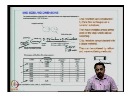
We will talk about surface mount device sizes and dimensions now. As you know, the chip resistors are constructed by thick film technique on a ceramic substrate; your resistors or your capacitors. They have metallic areas at the end of the chip like you have the surface mount devices; so at the end you will have the connector points. These are the metallic areas and here it could be the ceramic material with a well defined dielectric
