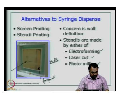
Now, we will look at alternatives to syringe dispense. Syringe can be used for both glue dispensing as well as any nonconductive glue, a conductive paste or a conductive adhesive or a solder paste. So, the applications are varied. Screen printing and stencil printing are the other methods that can be used to dispense materials or media. The concern here is the wall definition that means you have to generate these kinds of screens
