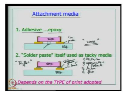
Now, let us look at some of the other processes typically that is used in a reflow soldering process. We must know about the attachment media. When a surface mount device whether it is an active device or a passive device, if it has to be attached to
