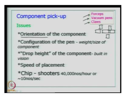
So, the idea is it should pick the components from the tape or the reel from which the packages are shift from the manufacturer and it has to pick individual components and place on the board based on your assembly data that you have generated from your PCB layout. So, the component pick up issues are; here we use forceps or vacuum pens or we also call it as Claws.
