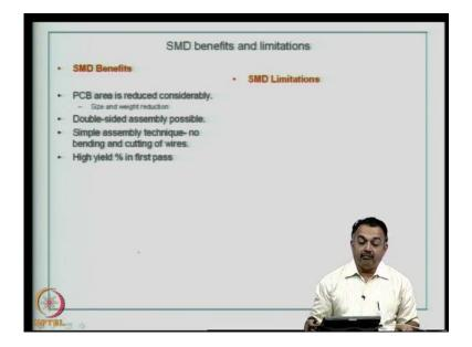
So, there are a wide variety of components that are available in surface mount format and if you are doing a re-engineering work, from a through-hole assembly into a surface mount assembly, then, you need to be aware of the packages that are available in the corresponding format. To begin with, let us look at the surface mount devices, benefits and limitations. Then you can compare this with the through-hole technology and try to see how a design can be ideally suited for such an assembly.
