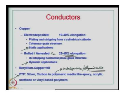
Conductor is essentially copper. It can be electrodeposited. We have seen the electrodeposition process – plating and stripping from a cylindrical cathode; you get a
