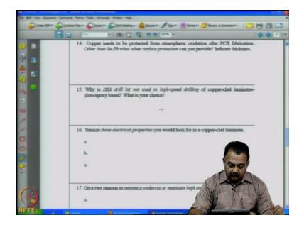
Copper needs to be protected from atmospheric oxidation after PCB fabrication. What other protection can you give other than tin-lead? You can use typically tin coating or the... lead is not being used today. You can ideally use nickel-gold. Nickel to the extent of 5 microns and gold to the extent of less than 1 micron can be used.
