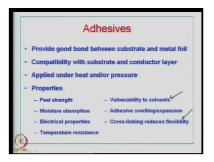
Adhesives are used to provide a good bond between the substrate and the metal foil; the dielectric and the metal foil. Compatibility should be there with the substrate and the conductor layer. It is applied under heat and pressure. So, it should bond well.
