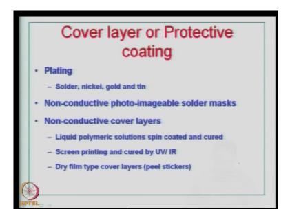
Cover layer or protective coating – either you can protect the copper with solder or nickel, gold, or tin; the similar thing that we have seen in rigid boards. Or, you can use non-conductive photo-imageable solder masks or non-conductive cover layers like a liquid polymeric solutions spin coated and cured, or it can be screen printed and cured by UV or IR, or it can be a dry film tape type of a material or a sticker type of material that can be easily applied and cured.
