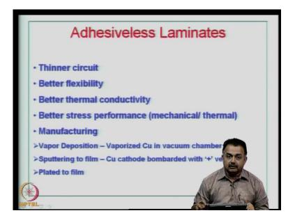
There are cases when we use adhesiveless structures, which mean you can reduce the thickness. So, you get a thinner circuit, better flexibility, better thermal conductivity, better stress performance, and the manufacturing is that you deposit the copper by using vapor deposition or sputtering process or simple electroplating directly on to the dielectric material.
