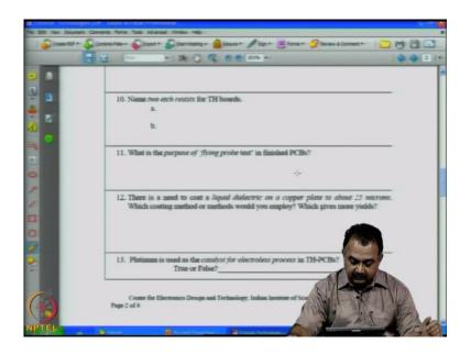
There is a need to coat a liquid dielectric on a copper plate to about 25 microns. Which coating method would you employ? For 25 microns, ideally you can use curtain coating or spin coating. Spin coating with good consistency can be achieved.
