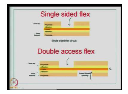
The cross-section of a single sided flex will be as shown here. We have discussed this before. You can access it from here. Now, a double access would mean that there is a single copper layer, but you can access from the top as well as from the bottom. After
