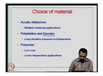
Choice of material: Acrylic adhesives – ideal for multiple soldering applications. Polyimides and epoxies – one would like to use epoxies because they are cost effective; long duration exposure to temperature is possible and you can see less defects with these kind of materials. Polyester is low cost and used for lower temperature applications. (Refer Slide Time: 41:43)
