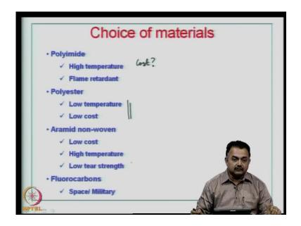
If you use a polyimide, as you know by now, ideally suited for high temperature; it is flame retardant, but at the same time, cost can be an issue. Then, polyester widely used in flex circuits – low temperature, low cost. Aramid non-woven structures – low cost, high temperature, low tear strength. Fluorocarbons ideally used for space and military.
