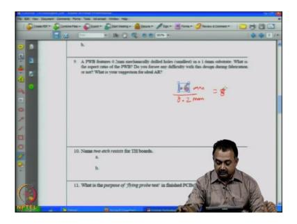
Now here there is a question about the aspect ratio. A PWB features 0.2 mm mechanically drilled holes in a 1.6 mm substrate. What is the aspect ratio of the PWB? I think we have discussed this in detail. So, 1.6 mm is the thickness and the drill size is 0.2 mm. So, the aspect ratio is 8.
