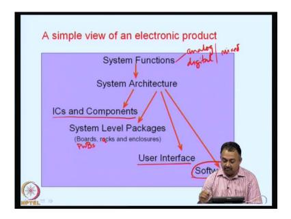
A simple view of an electronic product will be: there will be system functions built; the system functions can be, for example, analog, it can be digital, it can be a mixed signal or it can be high band width system function. It can be Radio Frequency, it can be optical or it can be mixture of each of these, depending on the application area.
