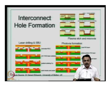
There is another method called wet etching, but it does not produce the kind of results that we expect; for this kind of high density interconnect structures using a dry plasma etch has been tried in prototyping, it produces better results in terms of the hole wall definition and the kind of undercut. When you talk about etching, there is always a problem with undercut and wet etching produces high undercut compared to dry plasma etch but, it is a very slow process.
