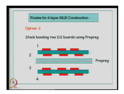
The second point using rigid laminates bonded with prepreg material. We are going to see both of these options. So, in the second case rigid laminates; let us see a 4-layer board is now introduced with two prepreg layers, one at the top and bottom and then you can have copper foil on both sides to get a 6-layer board. Let us look at the case study or an example for a 4-layer multilayer board construction.
