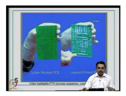
Now, the particular board has been solder masked, you can use a dry film or a liquid solder mask and then complete the operation. You can also see that the legend printing has been done on the right side; you can see legend print using white ink have been marked.
