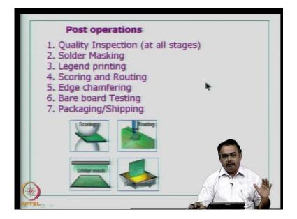
So this completes basically, the plated through hole process sequence for doing a double sided electrical interconnection. Now you can repeat these steps for multilayer board, but
