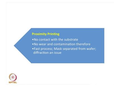
Proximity printing on the other hand, the next point that you see here, which is typically not used in the PCB industry today, but used in semiconductor industry were the mask will not touch the surface of the substrate. There will be a small gap, a very small gap typically about 15 microns to 20 microns gap between the mask and the substrate.
