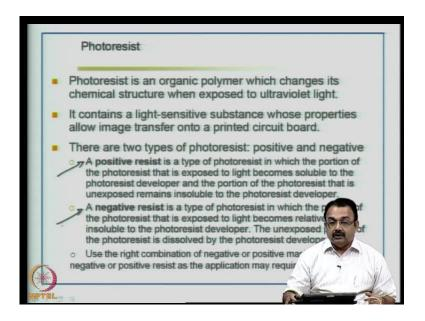
What is a photoresist? A photoresist is an organic polymer which changes its chemical structure when exposed to UV light. Our first job is to coat a photoresist and expose it to
