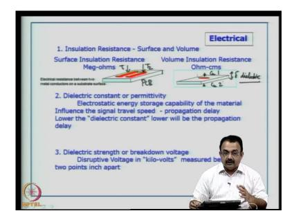
Electrical properties; we are interested in understanding insulation resistance, both surface and volume resistance. Surface insulation resistance is basically the electrical resistance between two metal conductors on a substrate surface. If you look at PCB like this and if you have two parallel tracks; tack one, track two let us say. We are interested in the electrical resistance that this material - dielectric material can provide.
