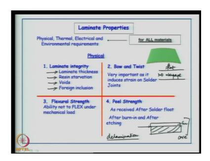
Now, we look at some of the laminate properties; we look at physical, thermal, electrical and environmental requirements. The physical properties and the laminate integrity are the properties that a manufacturer will check and pass it onto the consumer – end-n consumer. Laminate integrity; what does it mean? We are worried about the laminate thickness; if you say it is 1.6 mm there will be a tolerance, but the dimensions have to be maintained.
