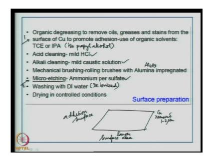
If you look at the copper clad laminate on the surface, you will see lot of organic grease. If you touch the copper clad laminate, your thumb impression or finger impression is going to be attached because your hand is greasy or because of the natural sweat or along
